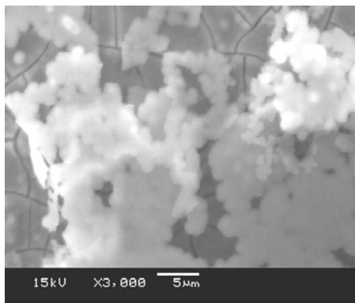
Fig. 7. SEM micrograph of surface layers on anodised samples of Ti in 2 M  $H_3PO_4$  after immersion for 192h in Ringer's solution at 298 K, mag x 3000
