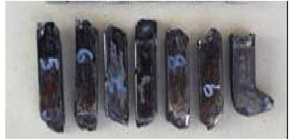
Fig.7. Steel samples after individual passes with use of the ECAP technology
