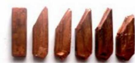
Fig. 2. Copper samples after individual passes with use of the ECAP technology
