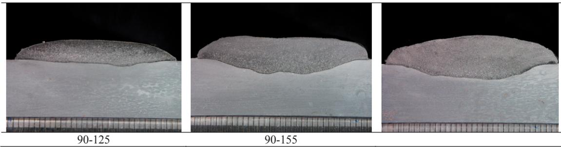
Fig. 1. Macrostructure of a single layer weave bead deposits produced with EnDotec DO\*11 wire of diameter 1,6 [mm]. Samples are marked - 65-125: 65 – torch inclination contrary to surfacing direction at an angle - 65° (push technique), 125 – arc current - 125 [A]
