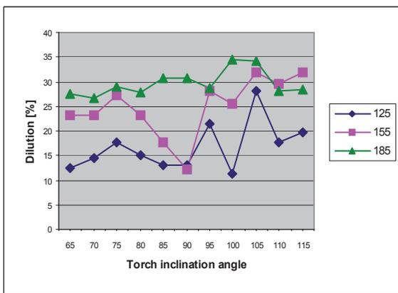
Fig. 2. Influence of arc current and the GMA torch inclination angle during robotized GMA surfacing with EnDotec DO\*11 wire of diameter 1,6 [mm], when weave technique applied, on dilution of the deposit - U
