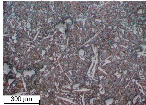
Fig. 4. Microstructure of the area under deposit's face of the third layer after GMA surfacing with EnDotec DO\*11 wire of diameter 1,6 [mm], stringer bead deposit– 95-3 and weave bead deposit – 185-3ww
