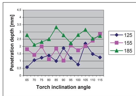
Fig. 3. Influence of arc current and the GMA torch inclination angle during robotized GMA surfacing with EnDotec DO\*11 wire of diameter 1,6 [mm], when weave technique applied, on penetration depth - hw
