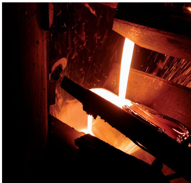
Fig. 1. A view of stone wool production process. Basalt lava is poured out from the ladle on the tapping spout from which is poured out to the cascade spinning rolls
