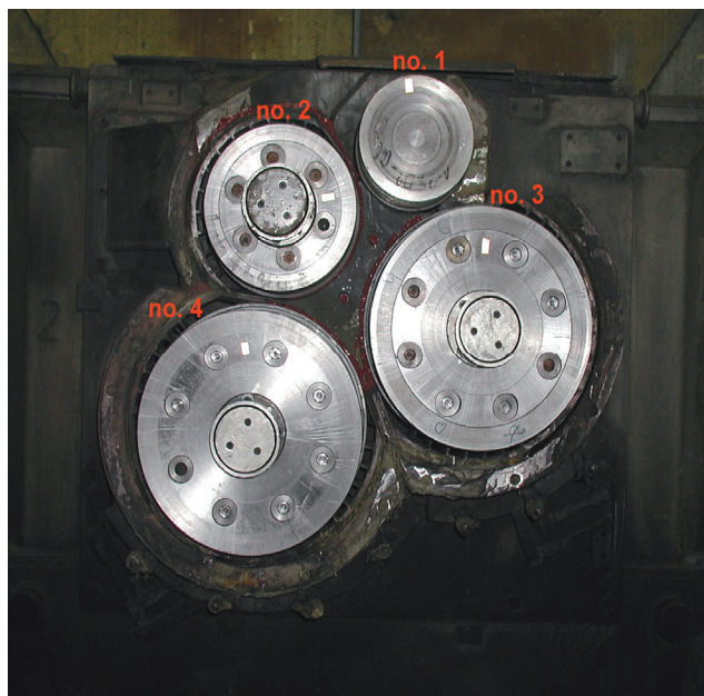
Fig. 2. A view of cascade spinning rolls of stone wool production apparatus of one company in Gliwice, Poland
