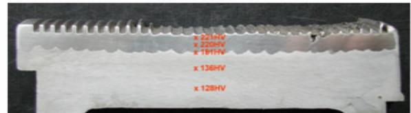
roll no 2, cross section – visible deep pits and hardness HV10
