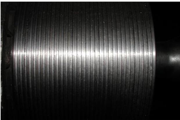
Fig. 1. A view of grooved working surface of spinning roll no 2. Grooved surface dimensions: groove width = 2,2 mm height of projection = 3,0 mm, width of projection = 1,5 mm
