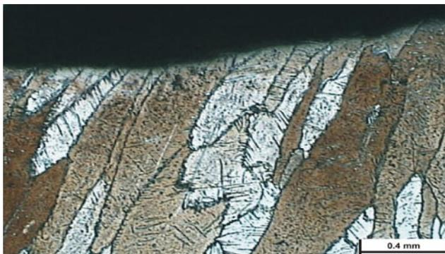
Fig. 6. Micrographs showing shape of a surface and microstructure of abrasion worn deposit of spinning roll No 3
