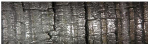
cracked surface of roll no 1
