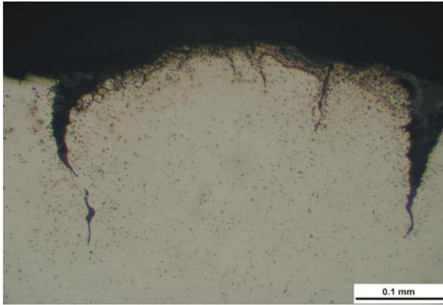
Fig. 4. Micrographs showing shape of a surface and fatigue cracks and fully austenitic microstructure of the corrosion-erosion and thermal fatigue worn spinning roll No 1
