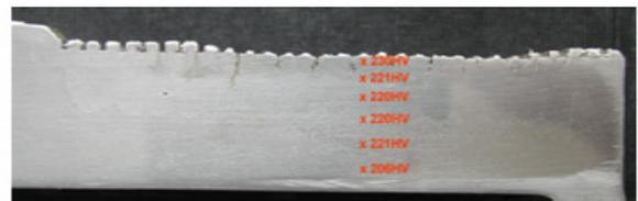
roll no 1, cross section – visible deep thermal fatigue cracks and hardness HV10
