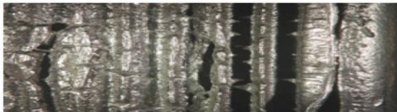
cracked surface of roll no 2
