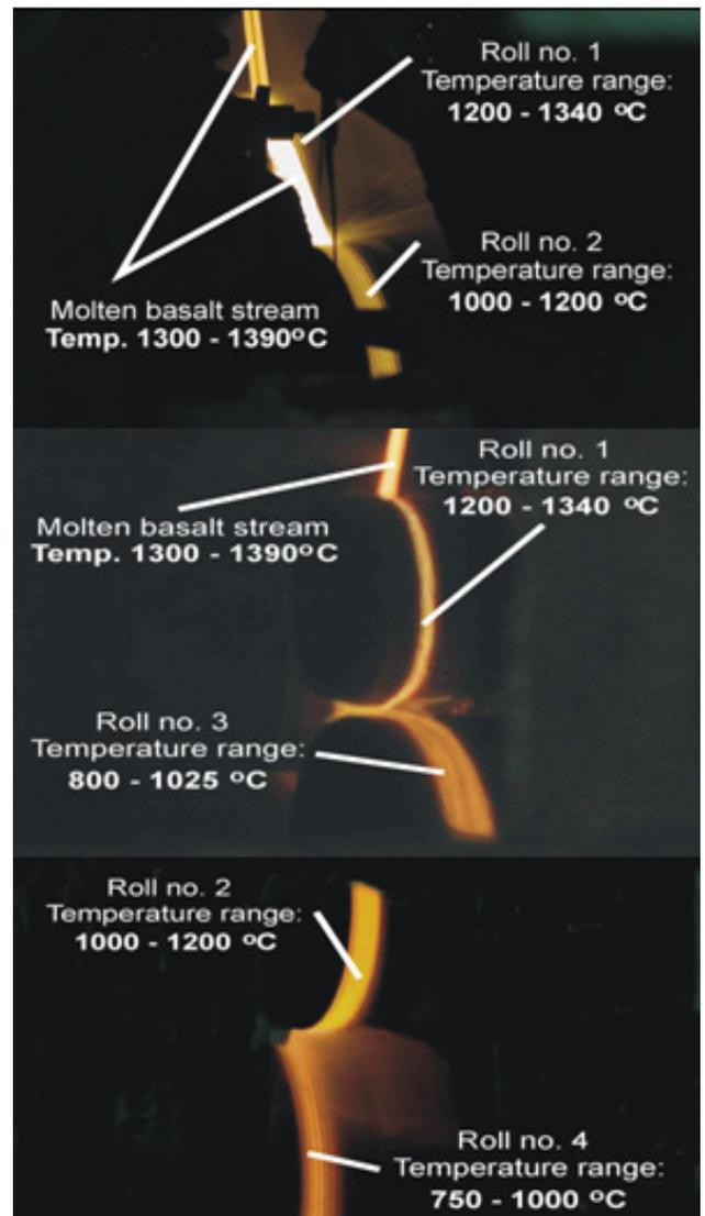
Fig. 2. Pictures of molten basalt lava stream impinging at working surface of spinning rolls and results of basalt lava temperature distribution measurements
