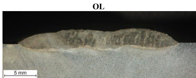
Fig. 3. Microstructure of single layer weave bead deposit of CASTOLIN 27 coated electrode MMA surfaced at (DC+) arc current 90 [A]
