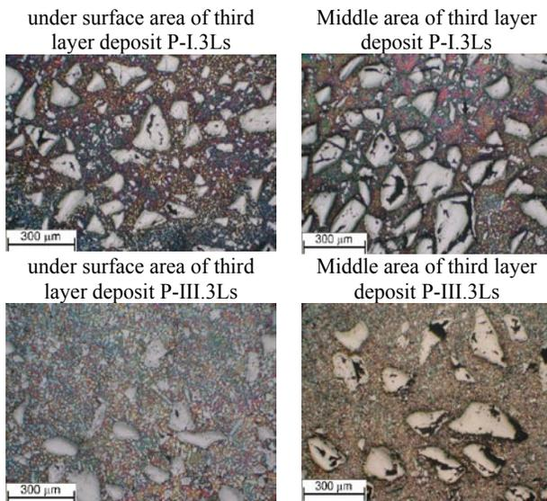
Fig. 4. Microstructure of third layer of deposits, Table 3, MCAW EnDOTec DO\*11 wire dia.1,6 [mm] surfaced
