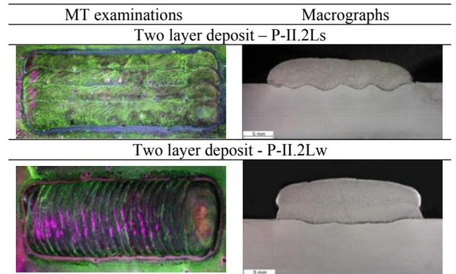
Fig. 2. A view of face during MT examinations and macrographs of two layers stringer and weave beads deposits. Table 3, MCAW EnDotecDO\*11 wire dia.1,6 [mm] surfaced
