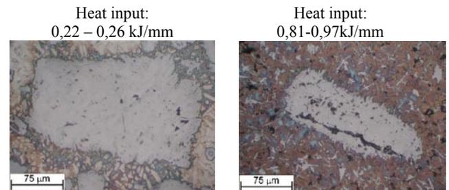
Fig. 3. Microstructure of tungsten carbides in stringer beads deposits surfaced with low and high heat input
