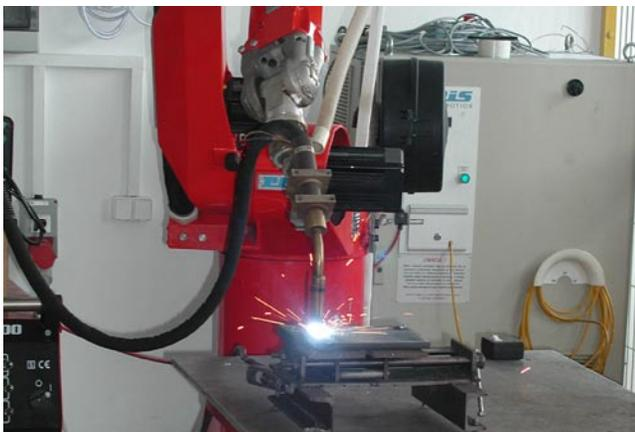
Fig. 1. A view of robotized stand for welding and surfacing equipped in programmable power source TotalArc<sup>2</sup> 5000 and REIS SRV6 welding robot
