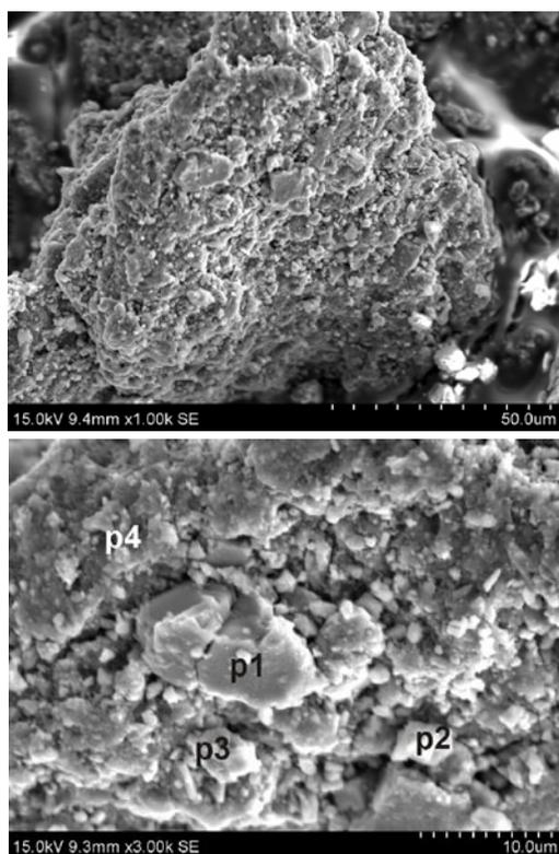
Fig.1. The image of the surface  $\text{AlFeTiO}_3$  composite powder after mechanical alloying process
