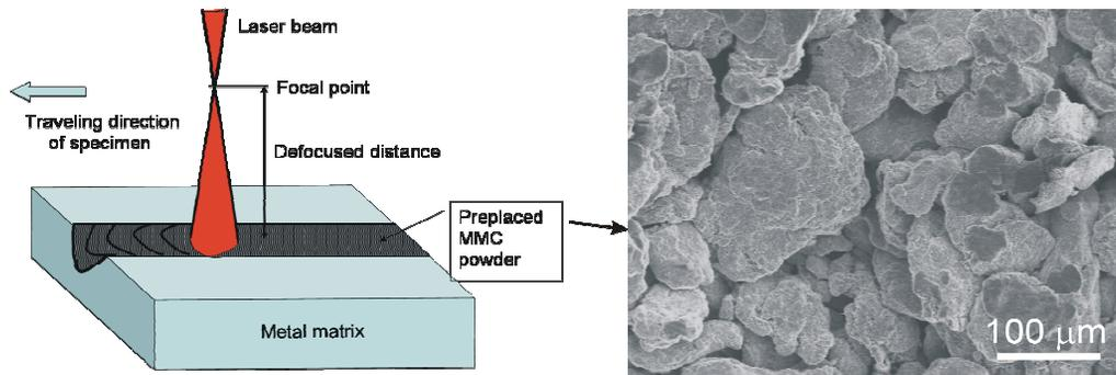
Fig.2. Schematic diagram of the CO<sub>2</sub> laser remelting geometry of the preplaced AlFeTiO<sub>3</sub> composite powder
