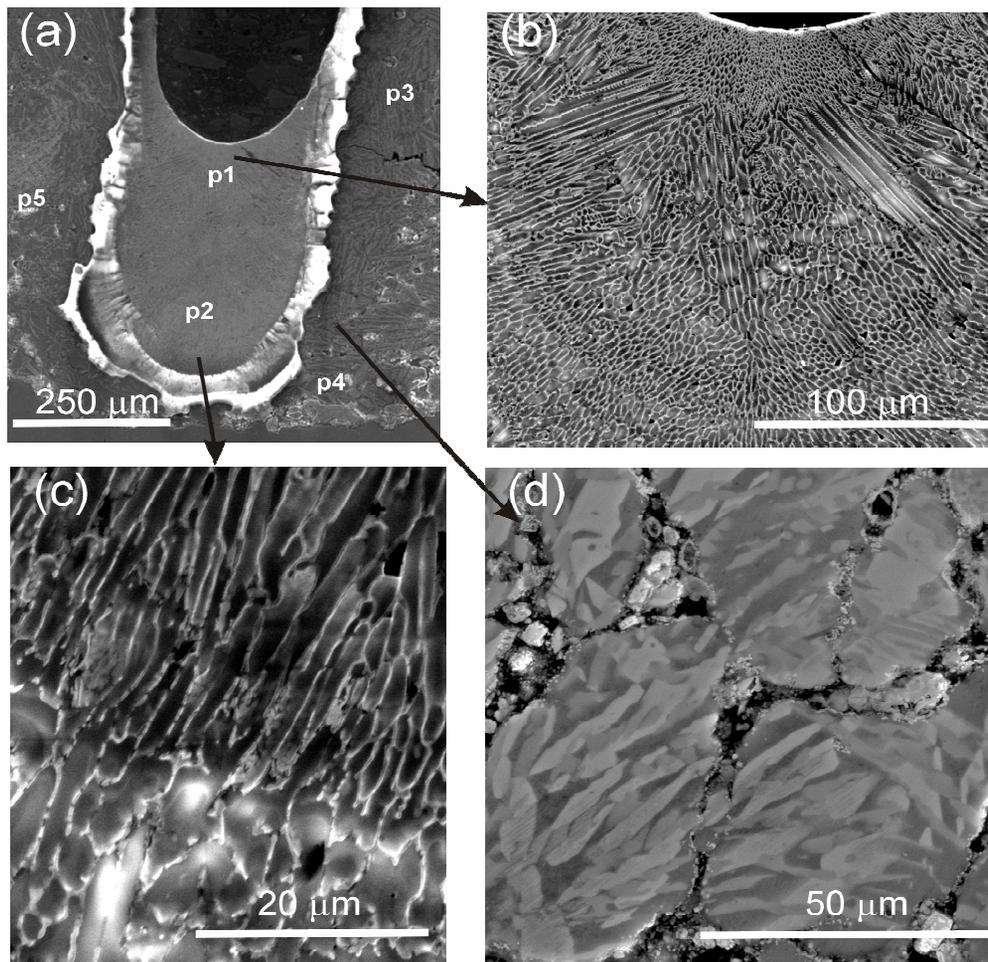
Fig.3. An SEM micrograph of the microstructure of the overall cross-sectional laser alloying AlFeTiO<sub>3</sub> composite powder incorporated in a aluminium matrix produced at  $10^5$  (W/cm<sup>2</sup>) laser energy density and 6,5 cm/s laser beam speed
