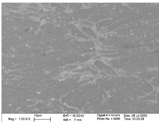
Fig. 5. Exemplary microstructure of deformed microcomposite with 3% wt. WC SEM
