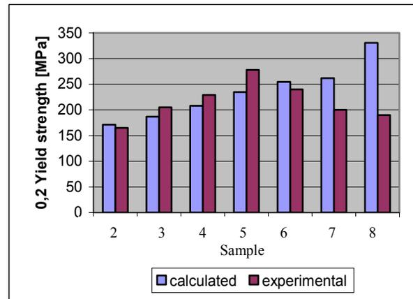
Fig. 3. Comparison of experimental and calculated values for the compressive 0.2% yield stress for the Cu micro-composites
