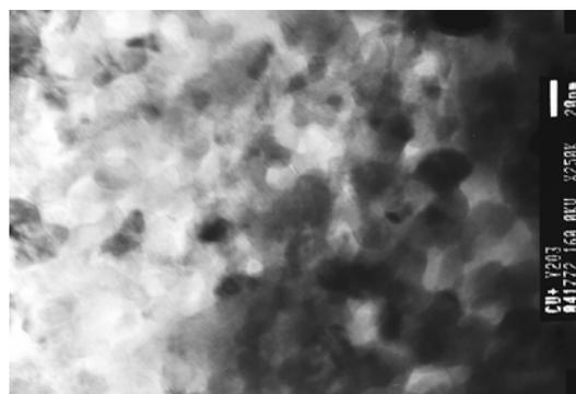
Fig. 2. Exemplary microstructure of the sintered nanocrystalline Cu - Y<sub>2</sub>O<sub>3</sub> micro-composite containing 2 wt.% of the hardening dispersoids; TEM
