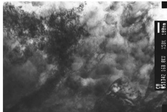
Fig. 4a. Microstructure of the deformed nanocrystalline copper; TEM
