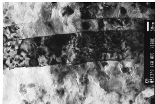
Fig. 4b. Microstructure of the deformed nanocrystalline copper; TEM
