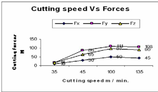
Fig.7. Cutting speed Vs Forces at 0.16 feed.
