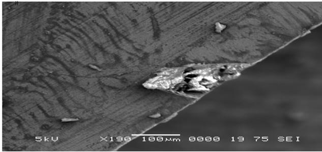
Fig.12. SEM view on micro cracks and chipping.
