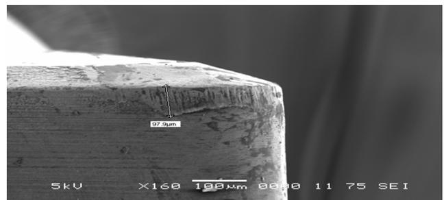
Fig 10 shows the flank wear and nose combined.
