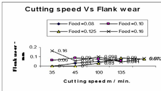
Fig.8. Cutting speed Vs flank wear.
