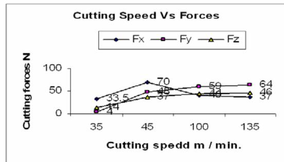
Fig. 5. Cutting speed Vs Forces at 0.10 feed.
