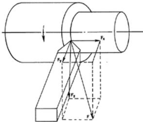
Fig.1. 3 Cutting forces acting on a tool.
