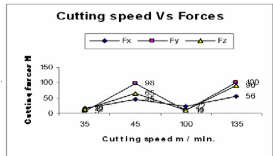
Fig.6. Cutting speed Vs Forces at 0.125 feed.
