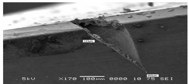
Fig.11. SEM view micro notch wear.
