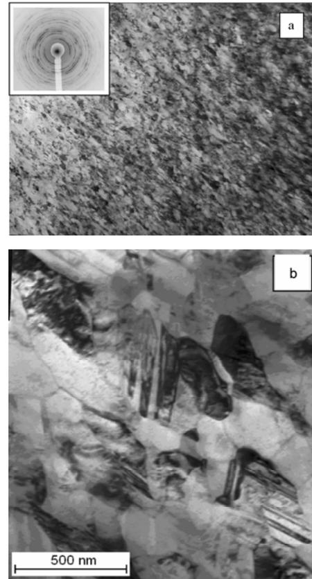
Fig. 3. The structure of buildup in the longitudinal direction: a – electron micrograph showing ultra-fine grains in buildup (x12.000, b – electron micrograph showing micro-twins inside very small grains (x60.000)
