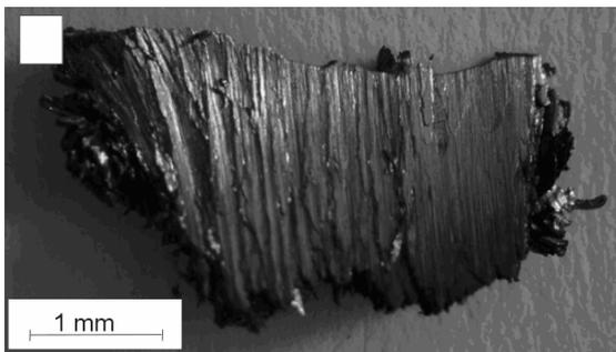
Fig. 2. Removed buildup
