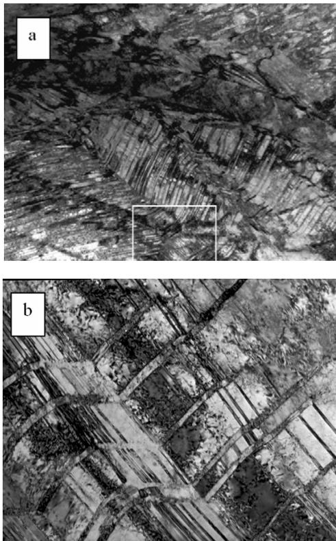
Fig.4. The buildup structure in transverse direction: a - electron micrograph (x12.000), b – electron micrograph of the another place taken at higher magnification (x35.000)
