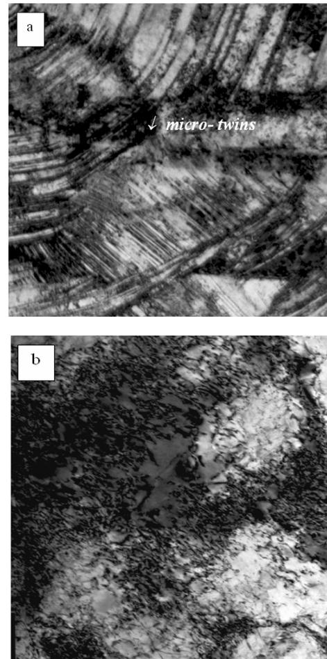
Fig.5. TEM micrograph of build up structure: a – the high magnification of micro - twins showed in fig.4a (total magn. x65.000), b – the region of showing high density dislocation structure in 1H18N9T stainless steel (x40.000), c – electron diffraction pattern with arrows showing the rings from martensite
