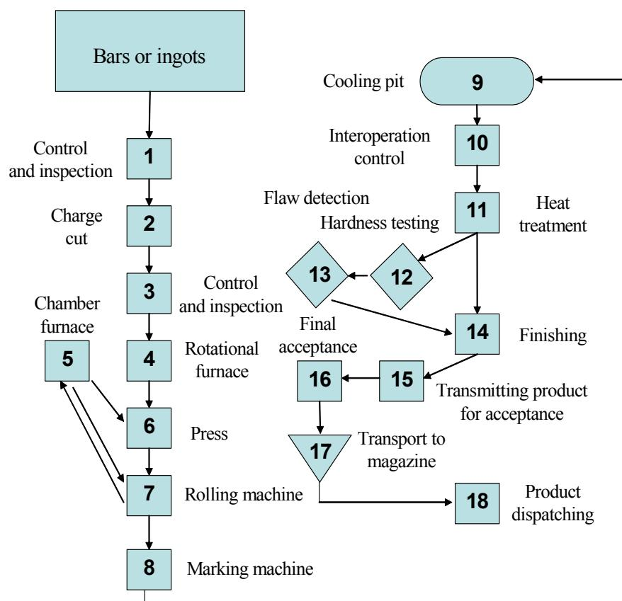
Fig. 1. The technological process of manufacturing the rings of train wheels [2]
