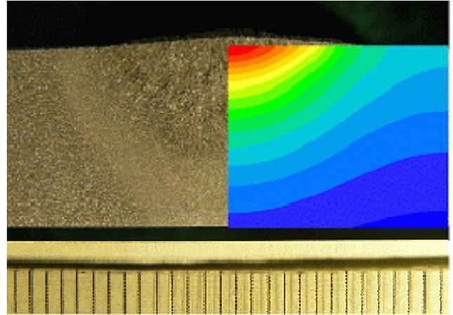
Fig. 4. Comparison of experimental and simulated results for Ar + 67% He shielding gas
