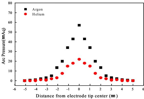
Fig. 3. The calculated results of the arc pressure on weldment surface for different types of shielding gas
