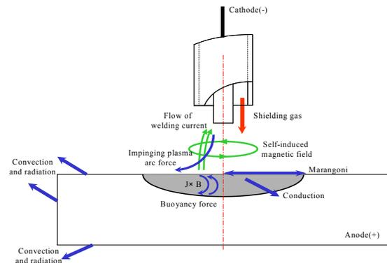
Fig. 1. A schematic diagram of the GTA welding process
