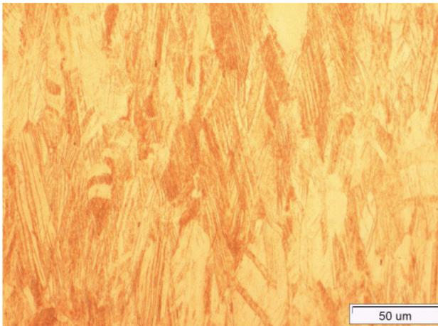
Fig. 6. Single – phase structure of bronze CuSn7 with sliding lines and deformation bands; tensile temp. 150°C, deformation zone of the sample; 500x
