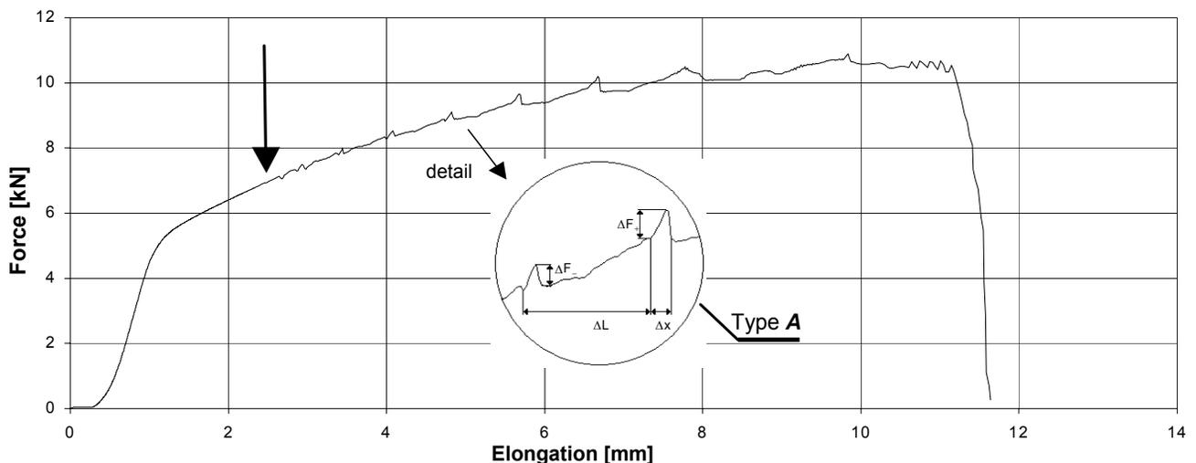
Fig. 1. Tensile stress-strain curve for CuSn7 alloy at 150°C
