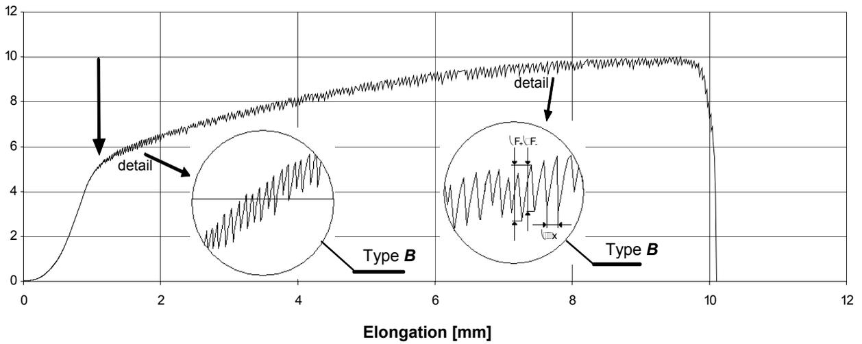
Fig. 2. Tensile stress-strain curve for CuSn7 alloy at 250°C
