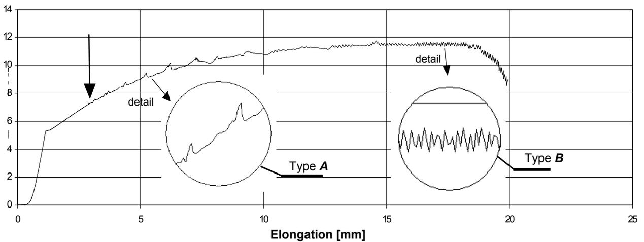
Fig. 4. Tensile stress-strain curve for CuSn7Zr0.01% alloy at 150°C
