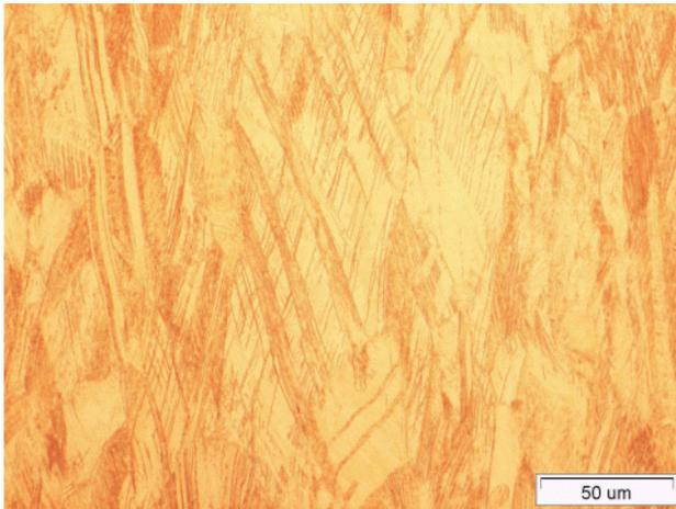
Fig. 5. Single – phase structure of bronze CuSn7 with the shear bands; tensile temp. 250° C, break–off zone of the sample; 500x
