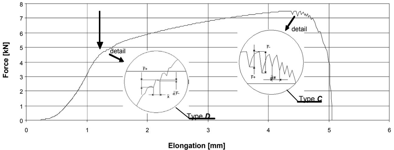
Fig. 3. Tensile stress-strain curve for CuSn7 alloy at 300°C
