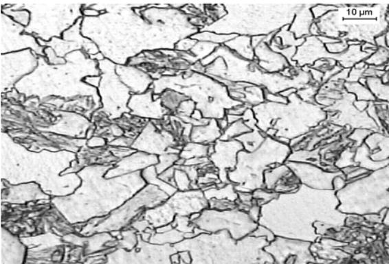
Fig. 4. Ferritic – martensitic structure of the steel quenched from a temperature of 750°C following air cooling for 45s from 910°C
