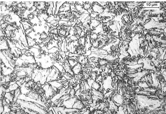
Fig. 3. Ferritic – martensitic structure of the steel twice quenched from the temperatures of 910°C and 750°C
