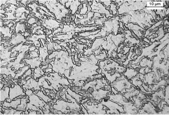
Fig. 2. Ferritic – martensitic structure of the steel quenched from a temperature of 750°C
