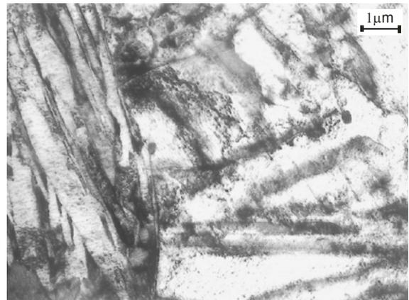
Fig. 5. Martensitic island in the ferrite matrix of high dislocation density
