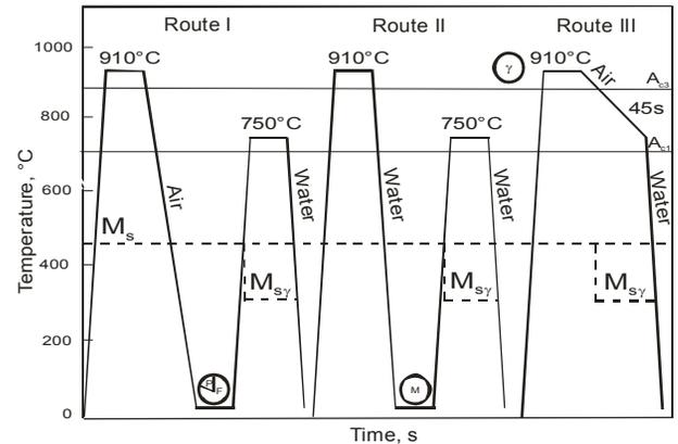
Fig. 1. Schematic representation of the heat treatment of DP-type steel according to routes I, II and III
