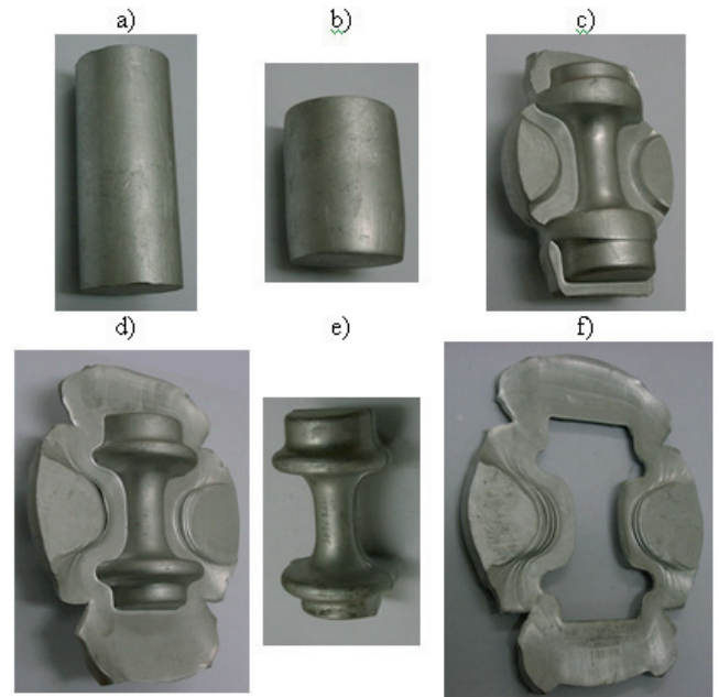
Fig. 2. Other phases of the wheel hub drop forging forming process on hammer: a) charge, b) upsetting, c) forging in preforming impression, d) forging in forming impression, e) final forged parts, f) flash
