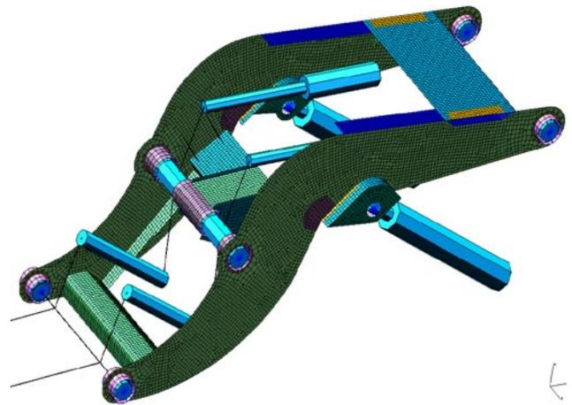
Fig. 3. Discrete model of the jib arm
