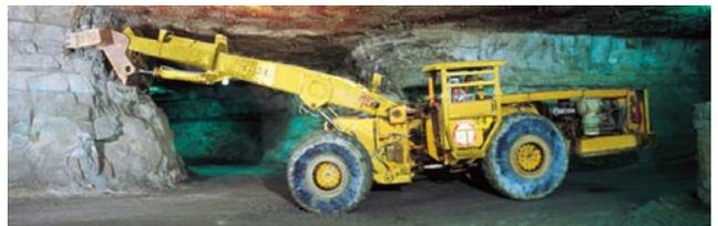
Fig. 1. SWB (Self-propelled roof ripping vehicles) during operation at an underground mine
