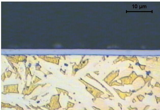
Fig. 2. Ti/CrN coating deposited onto the CuZn40Pb2 substrate
