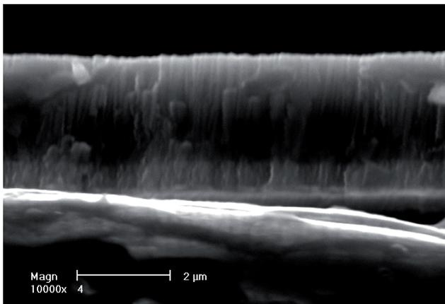
Fig. 3. SEM micrograph of fracture in Ti/TiAlN sample
