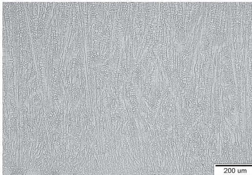
Fig. 1. The structure of the X40CrMoV5-1 hot work tool steel alloyed with TaC, scanning rate 0.5 m/min, power range 2.0 kW
