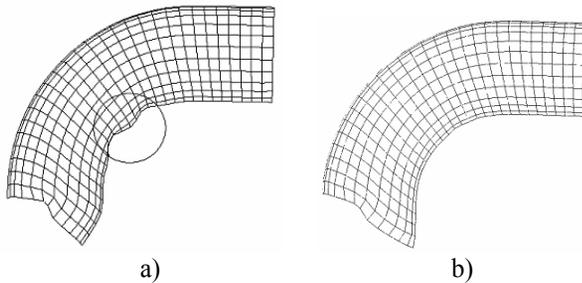
Fig. 6. Results for simulation of forming, a) with wrinkling, b) without wrinkling
