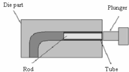
Fig. 1 Symbolic representation of experimental apparatus – before forming
