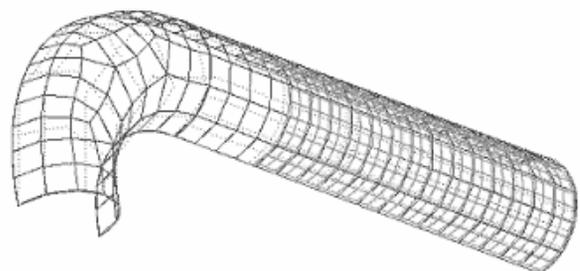
Fig. 4. FEM mesh of die and blank
