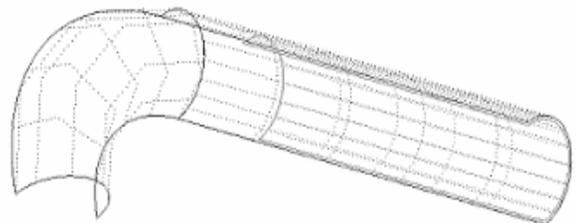
Fig. 3. FEM model of die and blank
