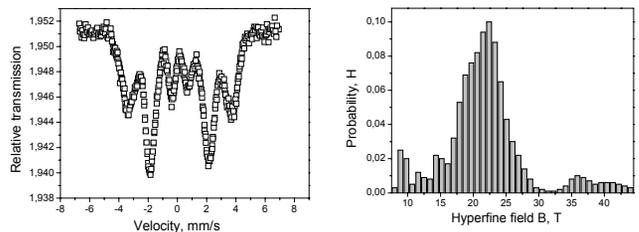
Fig. 1a The Mössbauer spectrum of the as quenched Co<sub>68</sub>Fe<sub>4</sub>Mo<sub>1</sub>Si<sub>13.5</sub>B<sub>13.5</sub> amorphous ribbon b) Distribution of the hyperfine fields P(H)
