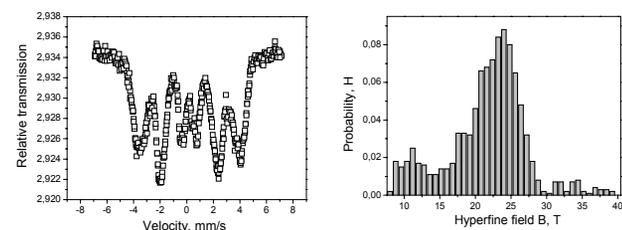
Fig. 5a. The Mössbauer spectrum of the powder obtained from the  $\text{Co}_{68}\text{Fe}_4\text{Mo}_1\text{Si}_{13.5}\text{B}_{13.5}$  amorphous strip annealed at the temperature of  $500^\circ\text{C}$  after 2 hours of milling, B) Distribution of the hyperfine fields P(H)
