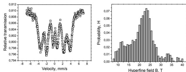
Fig. 4a. The Mössbauer spectrum of the powder obtained from the  $\text{Co}_{68}\text{Fe}_4\text{Mo}_1\text{Si}_{13.5}\text{B}_{13.5}$  amorphous strip after 25 hours of milling, b) Distribution of the hyperfine fields P(H)
