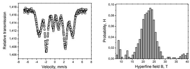
Fig. 2a. The Mössbauer spectrum of the Co<sub>68</sub>Fe<sub>4</sub>Mo<sub>1</sub>Si<sub>13.5</sub>B<sub>13.5</sub> amorphous strip annealed at the temperature of 500°C, b) Distribution of the hyperfine fields P(H)
