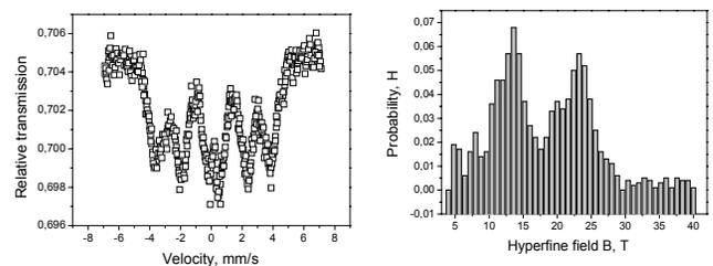
Fig. 3a. The Mössbauer spectrum of the powder obtained from the Co<sub>68</sub>Fe<sub>4</sub>Mo<sub>1</sub>Si<sub>13.5</sub>B<sub>13.5</sub> amorphous strip after 15 hours of milling, b) Distribution of the hyperfine fields P(H)
