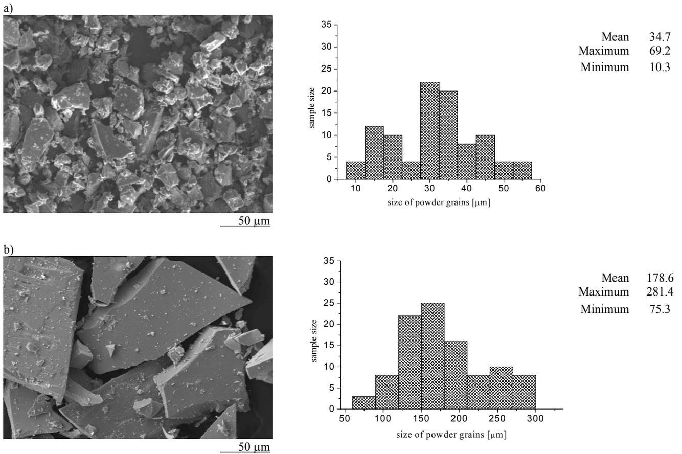
Fig. 2. Morphology, distribution and comparison of powders particle size of: a)  $Fe_{73.5}Cu_1Nb_3Si_{13.5}B_9$ , b)  $Nd_{14.8}Fe_{76}Co_{4.95}B_{4.25}$
