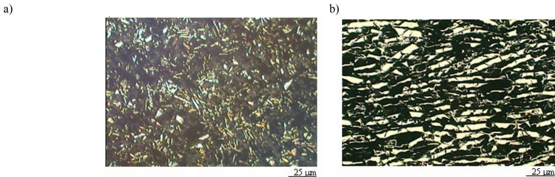
Fig. 3. Topography of the surface of composite materials: a) FINEMET – PEHD b) Nd-Fe-B – EP
