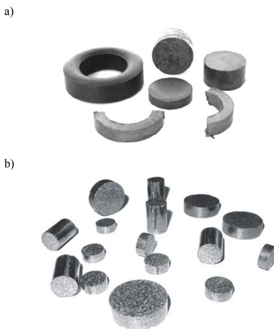
Fig.1. Composite materials: a) FINEMET – PEHD b) Nd-Fe-B – EP
