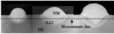
Fig. 2. Optical macrographs through welded section of Sample 2 showing: parent metal, PM, weld metal, WM, and heat affected zone, HAZ
