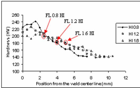
Fig. 3. Hardness profiles 1.5 mm below the surface of the parent material from the center line of the weld  $x = 0$ , showing fusion line (FL) for three samples.
