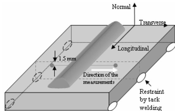
Fig. 1. Illustration of fully restrained single bead-on-plate, showing the direction of the measurements (transverse x, normal y, longitudinal z) using neutron diffraction
