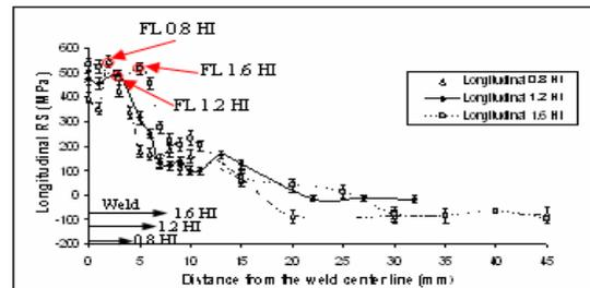
Fig. 5. Longitudinal residual stresses measured by ND against distance from the weld center line. Error bars based on uncertainty in the value of the peak diffraction angle are shown.
