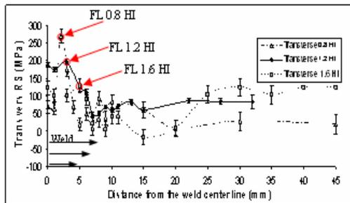
Fig. 6. Transverse residual stresses
