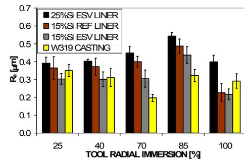
Fig. 5. Arithmetic average roughness ( $R_a$ ) of the machined surface for the three (3) Al-Si liner types investigated, as well as the W319 machined surface, versus the percentage of the tool radial immersion. Standard deviations are as indicated
