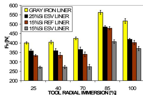
Fig. 4. Resultant cutting force ( $F_R$ ) versus the percentage of the tool radial immersion for the three (3) Al-Si liner types investigated, as well as the gray iron liner commonly used in the industry. Standard deviations are as indicated
