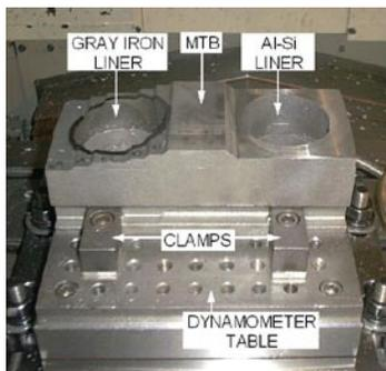
Fig. 2. Setup for the MTB HSM showing the MTB mounted on a Kistler 9255B type dynamometer table used for on-line cutting force measurements
