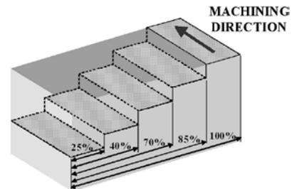
Fig. 3. A schematic representation of the tooling immersions used in this study
