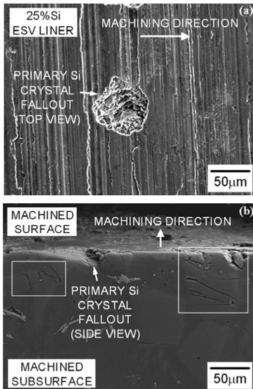
Fig. 8. SEM/SE micrographs of the 25%Si ESV liner machined surface showing two views: (a) top machined surface view, and (b) polished cross-sectioned side view
