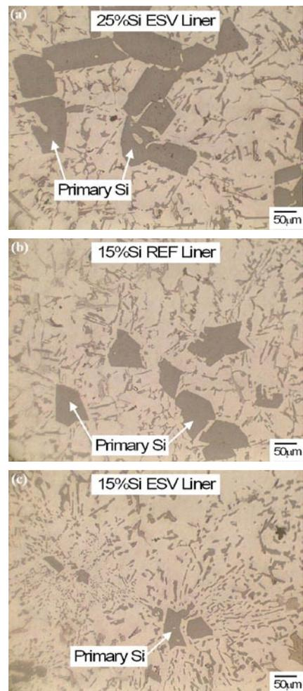
Fig. 7. Primary Si particle size comparisons between the three Al-Si liner types investigated
