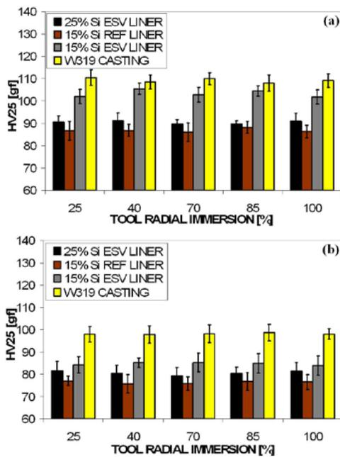
Fig. 6. Aluminum matrix microhardness (HV25) of the machined subsurface matrix structure (a), and the bulk material matrix structure (b) Al-Si cast liner structures for the three (3) investigated liner types, and the W319 cast matrix. Standard deviations are as indicated
