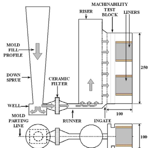
Fig. 1. A schematic diagram of the Machinability Test Block (MTB) casting mold showing the cross-sectional side view of the sand mold package along with the mold fill profile, and the cross-sectional top view of the mold package (MTB dimensions are in millimeters)
