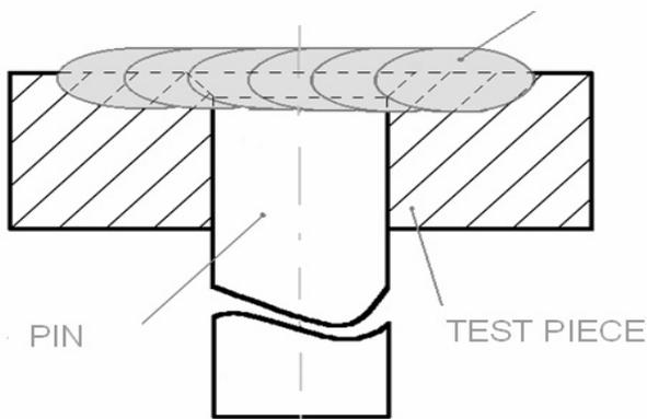
Fig. 6. Dimensions and view of the implant test after surfacing
