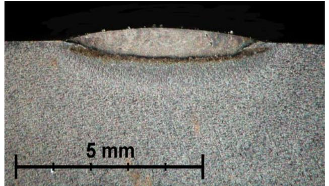
Fig.4 Padding weld macrostructure (No 4), laser beam power 1.2 [kW], powder flow rate 3.8 [g/min], Tables 3 and 4
