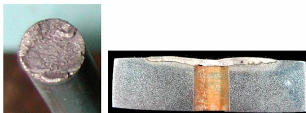
test piece broken in the area of padding weld fusion with the pin face surface
