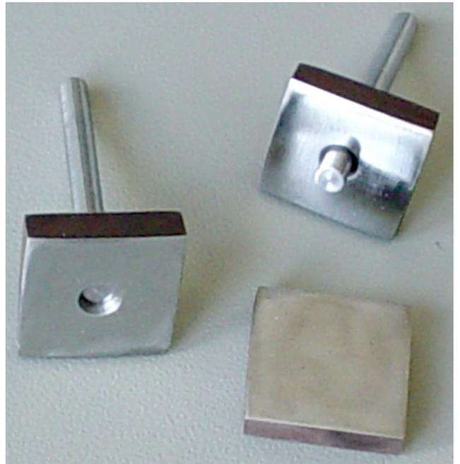
Fig. 8. Test pieces prepared for laser powder surfacing for adhesion tests of the padding weld to the substrate
