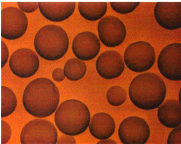
Fig. 3. Granules of EuTroLoy 16223 powder, magnification 300 ×
