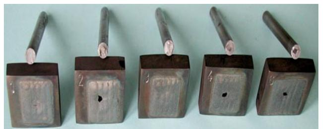
Fig. 10. Pin test pieces after adhesion test Holes visible in padding welds pulled out with the pin
