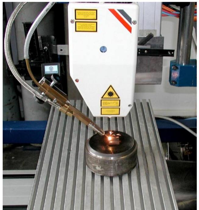
Fig. 2. Stand for laser surfacing and for the laser surfacing of the test plate: A – HPDL DL020 laser head, B – NC controlled table, C – control computer, D – concentric powder feed and shield gas nozzles, E – transport gas (argon) cylinder, F – shield gas (argon) cylinder
