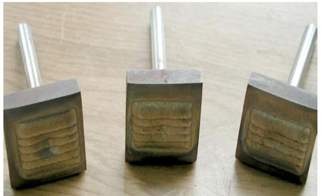
Fig. 9. Pin test pieces after laser powder surfacing
