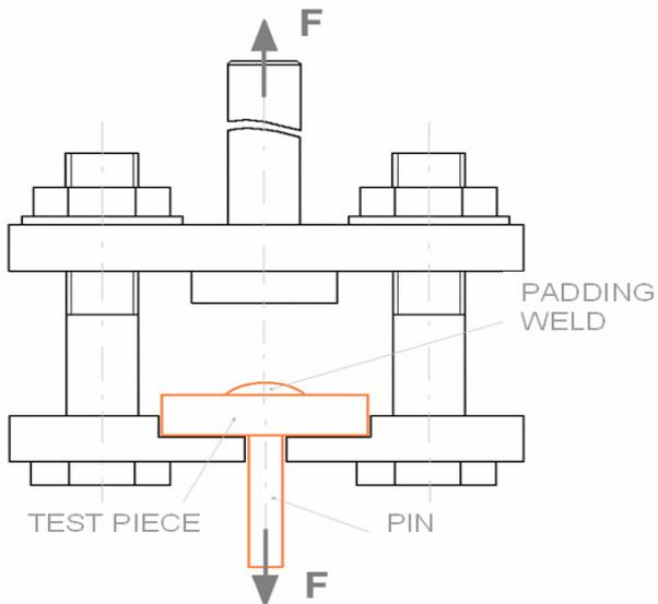
Fig. 7. View of the device for static tensile test of the pin test piece, Fig. 6
