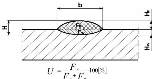
Fig. 1. Portion of the substrate material in padding weld, where:  $H_n$  – padding weld height,  $H$  – padding weld thickness,  $H_w$  – fusion penetration depth,  $b$  – padding weld width,  $U$  – portion of substrate material in padding weld [%],  $F_w$  – fusion penetration surface area,  $F_n$  – padding weld surface area
