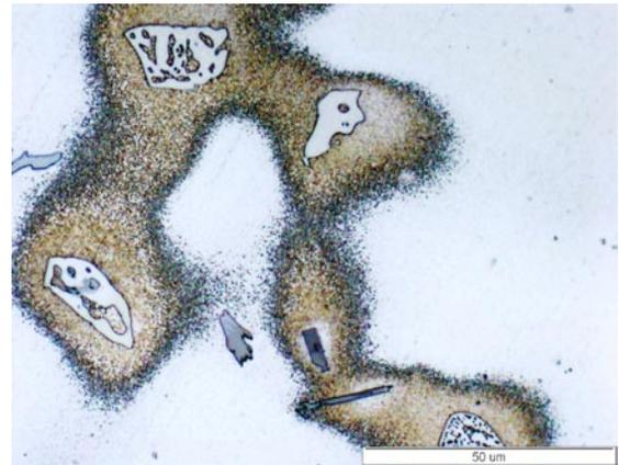
Fig. 1. LM microstructure of as-cast AE42 alloy
