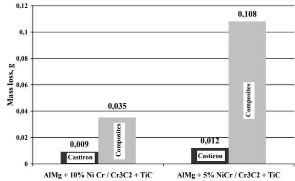
Fig. 5. The loss of cast iron counter sample mass after collaboration in dry sliding conditions at the 5000m distance
