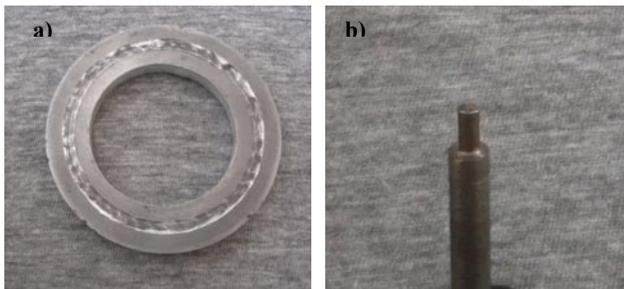
Fig. 4. View of the frictional couple cast iron- AIMg+5% NiCr/Cr<sub>3</sub>C<sub>2</sub>+TiC composite: a) composite ring, b) cast iron pin
