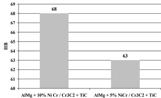
Fig. 6. The hardness of HB Composites layers under the process of wear
