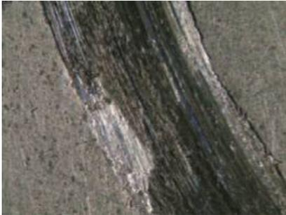
Fig. 8. Erosion rack on the AlMg+5% NiCr/Cr<sub>3</sub>C<sub>2</sub>+TiC composite layer, mag. 50x
