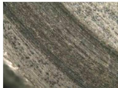
Fig. 7. Erosion rack on the AIMg+10%NiCr/Cr<sub>3</sub>C<sub>2</sub>+TiC composite layer, mag. 50x
