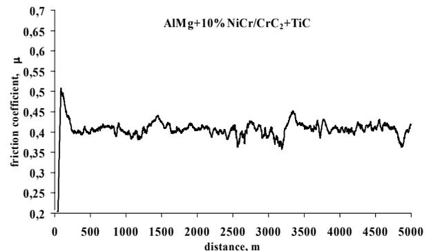
Fig. 1. The diagram of friction coefficient shifts in track function for AlMg+10% NiCr/Cr<sub>3</sub>C<sub>2</sub>+TiC composite
