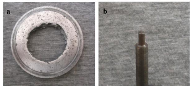
Fig. 2. View of the frictional couple cast iron- AlMg+10% NiCr/Cr<sub>3</sub>C<sub>2</sub>+TiC composite: a) composite ring, b) cast iron pin
