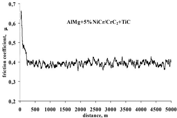
Fig. 3. The diagram of friction coefficient shifts in track function for AIMg+5% NiCr/Cr<sub>3</sub>C<sub>2</sub> + TiC composite
