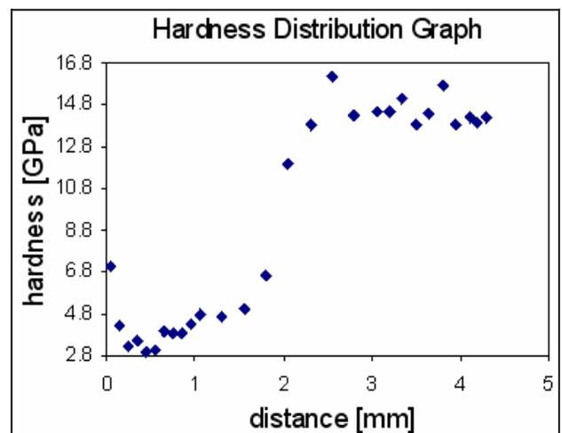
Fig. 4. The hardness *HV0.5* distribution in the cermet with graded microstructure; material was prepared by the centrifugal deposition method
