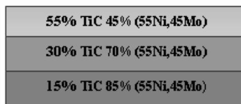
Fig. 1. Scheme of TiC – mixture (Ni, Mo) material with the phases content gradient, prepared by the layers pressing method
