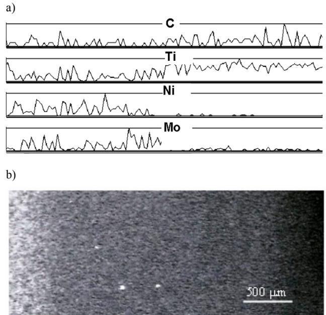
Fig. 3a). Elements: C, Ti, Ni, Mo distributions in cermet with the gradient of phases content; 3b) Microstructure of the graded cermet
