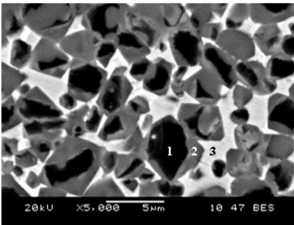
Fig. 2. Microstructures of the TiC-(Ni,Mo) cermet after sintering at vacuum atmosphere: 1) TiC grain (black colour), 2) (Ti,Mo)C ring (gray colour) and 3) Ni-Mo matrix
