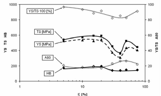
Fig. 2. Mechanical properties of samples annealed by mode 2
