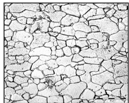
Fig. 11. Annealing mode 3, deformation 75 %
