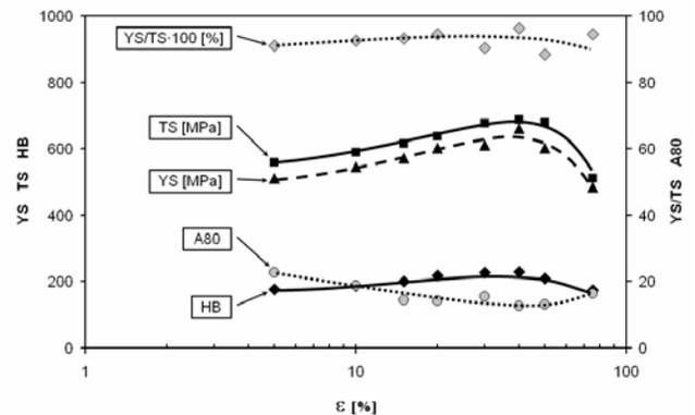
Fig. 1. Mechanical properties of samples annealed by mode 1
