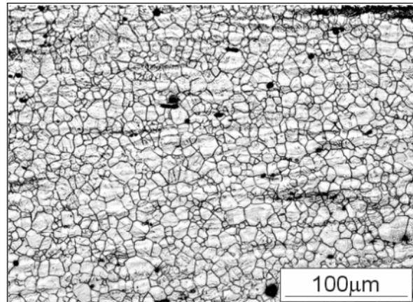
Fig. 5. Specimen A6 after annealing 850°C/0.5h, LM micrograph of metallographic sample after electrolytical etching.
