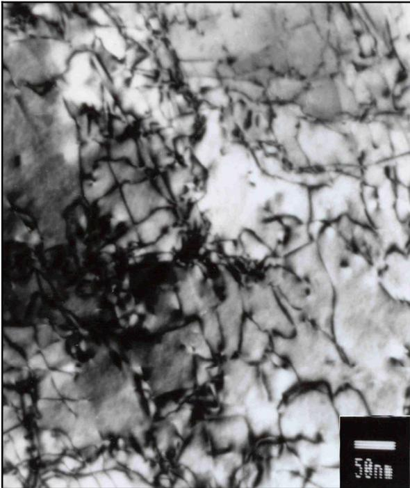
Fig. 2. Central part of specimen A6. TEM micrograph of thin foil. Strained austenite grain with a high dislocation density.
