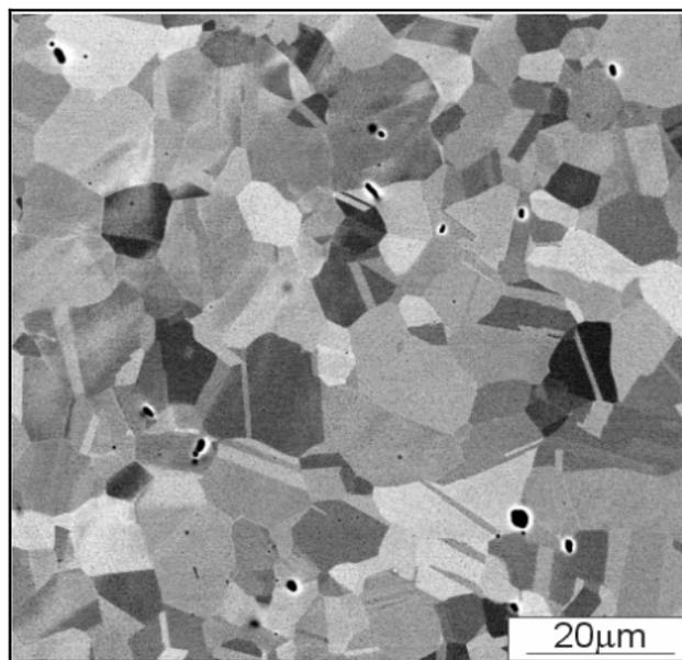
Fig. 6. Specimen A6 after annealing at 850°C / 0.5h. SEM micrograph – backscattered electron image of metallographic sample after electrolytic polishing.
