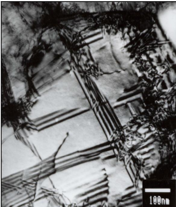
Fig. 3. Central part of specimen A6. TEM micrograph of thin foil. Strained austenite grain with deformation twins.
