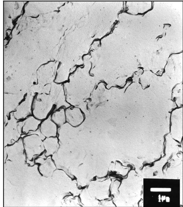
Fig. 4. Partly recrystallized structure of specimen A6. TEM micrograph of extraction carbon replica. Large strained and small recrystallized grains.
