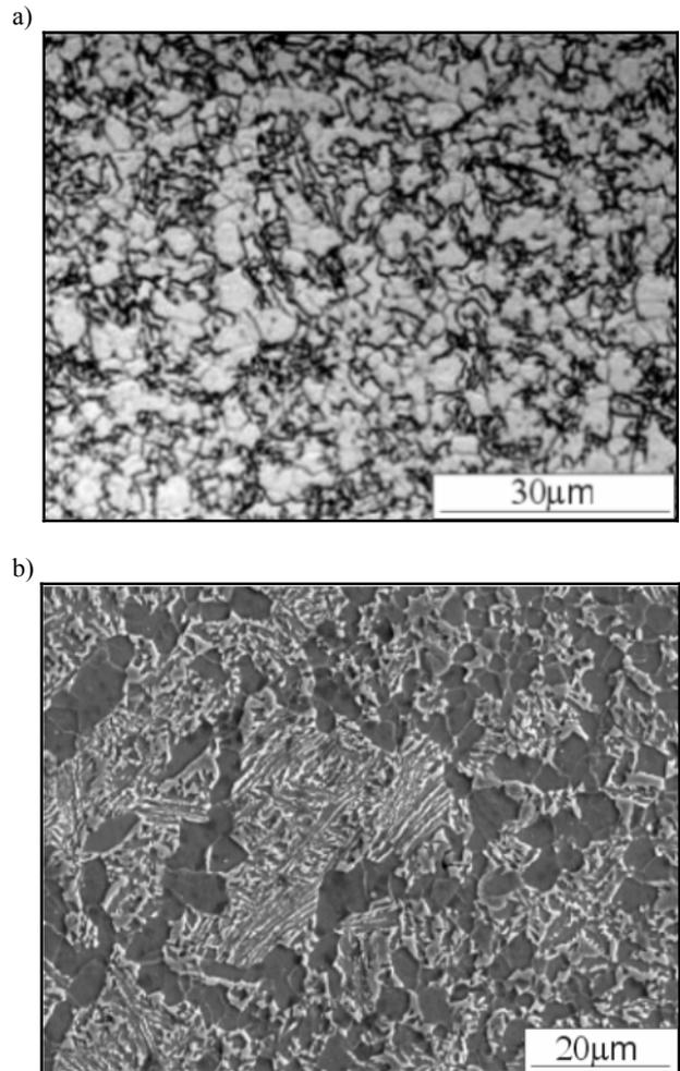
Fig. 8. Rim part of specimen T1, metallographic sample, colour etching: (a) LM micrograph, (b) SEM micrograph – secondary electron image.
