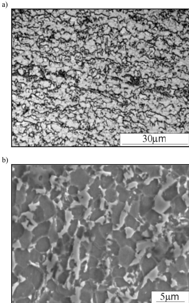
Fig. 7. Central part of specimen T1, metallographic sample, colour etching: (a) LM micrograph, (b) SEM micrograph – secondary electron image.
