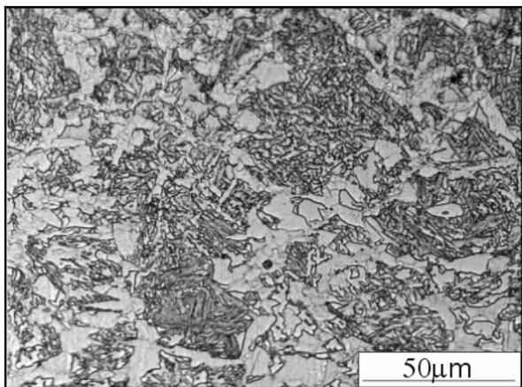
Fig. 10. Rim of specimen T3, LM micrograph of metallographic sample etched in nital.
