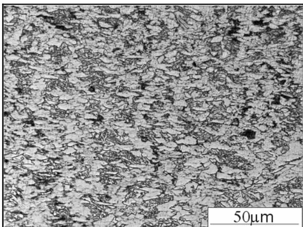
Fig. 9. Central part of specimen T3, LM micrograph of metallographic sample etched in nital.
