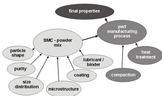
Fig. 2. Factors affecting on final SMC properties [1]
