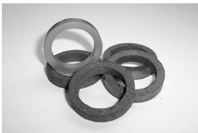
Fig 3. Soft magnetic composites based on nanocrystalline  $Fe_{73.5}Cu_1Nb_3Si_{13.5}B_9$  and Fe powders
