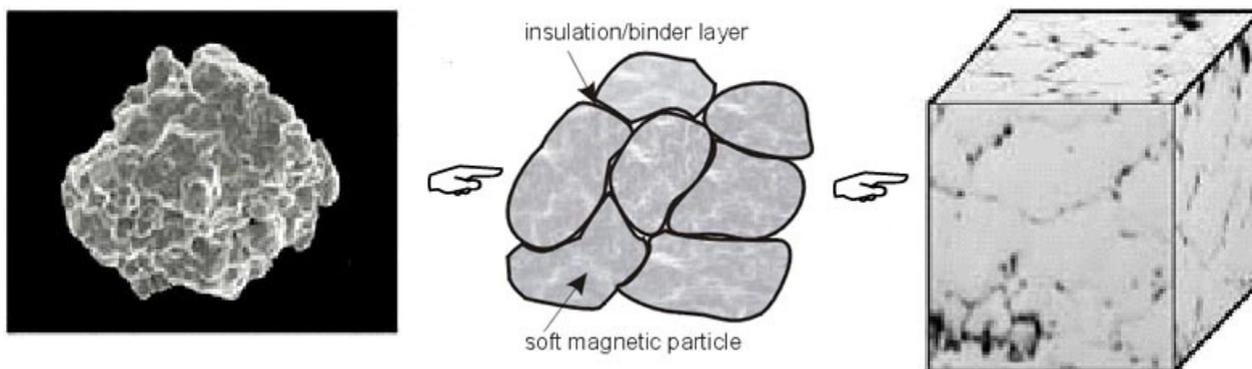
Fig. 1. Composition and processing of soft magnetic composite [2]
