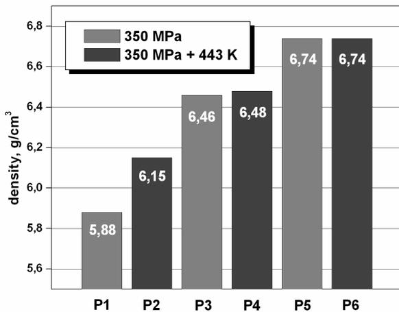
Fig. 4. The average densities of soft magnetic composites with different volume fraction of  $\text{Fe}_{73,5}\text{Cu}_1\text{Nb}_3\text{Si}_{13,5}\text{B}_9$  and Fe powders.
