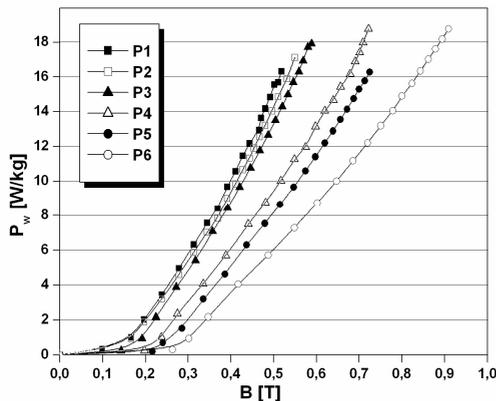
Fig. 10. The core losses as a function of magnetic induction of soft magnetic composites with different powder fraction.
