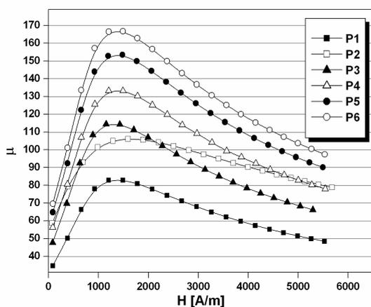
Fig. 8. The permeability as a function of applied magnetic field of soft magnetic composites with different powder fraction.
