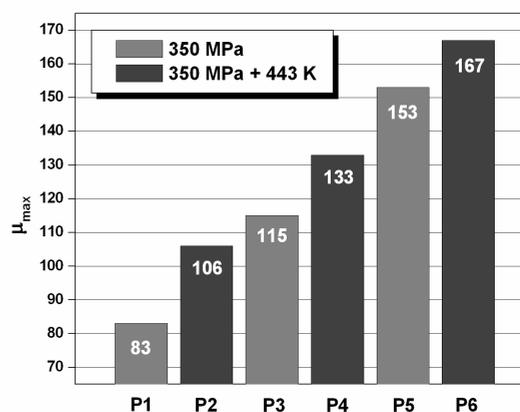
Fig. 9. The permeability of soft magnetic composites with different volume fraction of  $\text{Fe}_{73.5}\text{Cu}_1\text{Nb}_3\text{Si}_{13.5}\text{B}_9$  and Fe powders.
