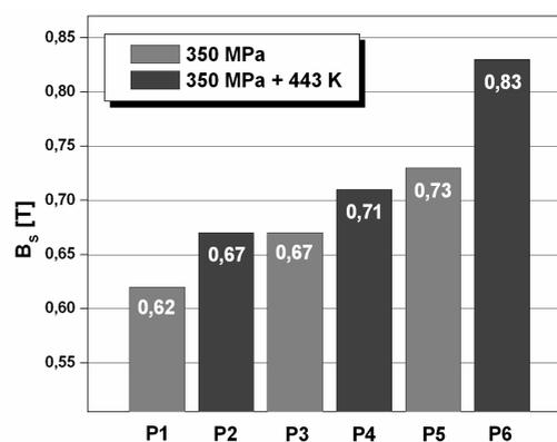
Fig. 7. The saturation induction of soft magnetic composites with different volume fraction of  $\text{Fe}_{73.5}\text{Cu}_1\text{Nb}_3\text{Si}_{13.5}\text{B}_9$  and Fe powders.
