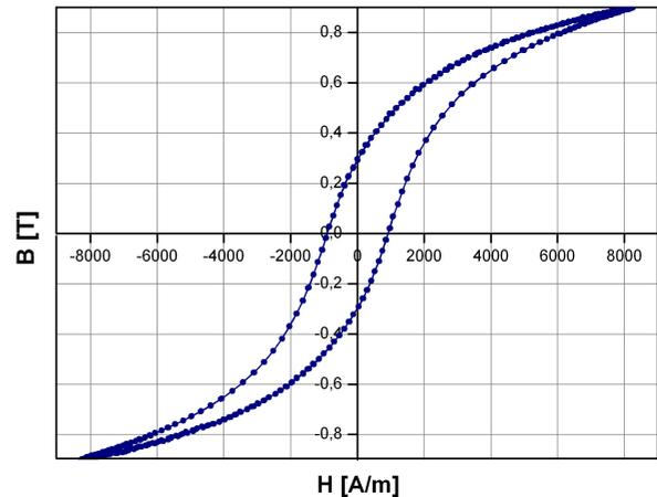
Fig. 5. Hysteresis loop for soft magnetic composite P6 obtained by compaction under pressure of 350MPa at 443 K.
