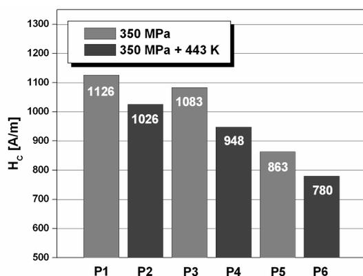
Fig. 6. The coercive field of soft magnetic composites with different volume fraction of  $\text{Fe}_{73.5}\text{Cu}_1\text{Nb}_3\text{Si}_{13.5}\text{B}_9$  and Fe powders.
