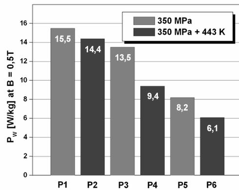
Fig. 11. The core losses of soft magnetic composites with different volume fraction of  $\text{Fe}_{73,5}\text{Cu}_1\text{Nb}_3\text{Si}_{13,5}\text{B}_9$  and Fe powders.
