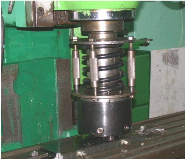
Fig. 3. The milling machine with the burnishing rotation head
