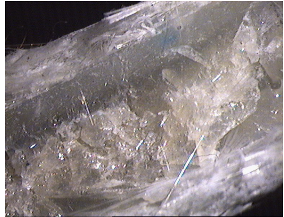
Fig. 8. Surface on the recyclate particle - matrix boundary fracture
