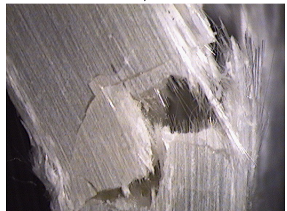
Fig. 9. Destruction on the recyclate - matrix boundary as a result of fracture and fibres pulling out
