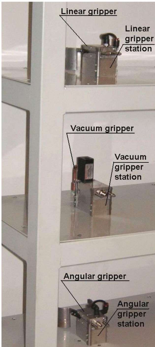
Fig. 11. Photography of all grippers' stations system
