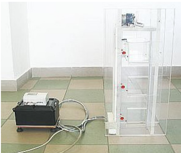
Fig. 10. The overall view of the lift's model. The shaft on the right and control unit on the left side.
