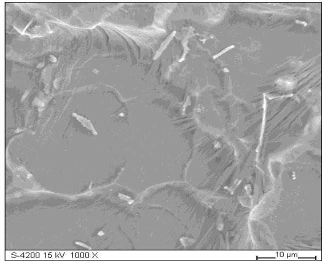
Fig. 7. Surface of Fe42Al alloy after corrosion tests in 3% H<sub>2</sub>SO<sub>4</sub> solution, scanning electron microscope, magn. 1000x.
