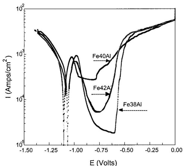
Fig. 1. Potentiodynamic curves in 0.2% HCl solution.
