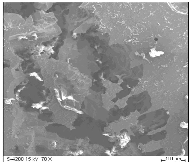
Fig. 8. Surface of Fe42Al alloy after corrosion tests in 0.2% HCl solution, scanning electron microscope, magn. 70x.
