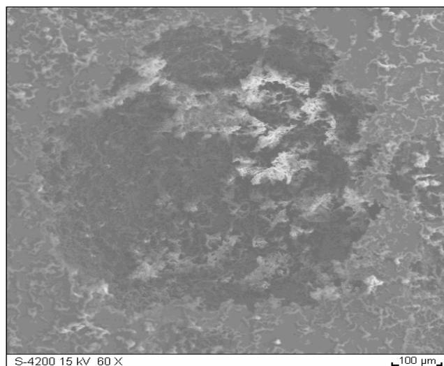
Fig. 4. Surface of Fe38Al alloy after corrosion tests in 0,2% HCl solution, scanning electron microscope, magn. 60x.
