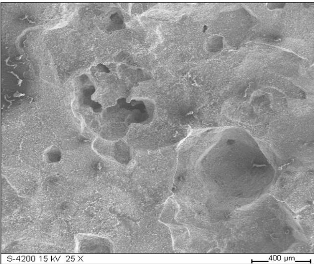
Fig. 6. Surface of Fe40Al5Cr alloy after corrosion tests in 0,2% HCl solution, scanning electron microscope, magn. 50x.
