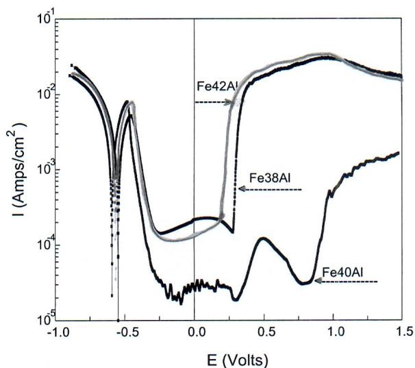
Fig. 2. Potentiodynamic curves in 3% H<sub>2</sub>SO<sub>4</sub> solution.
