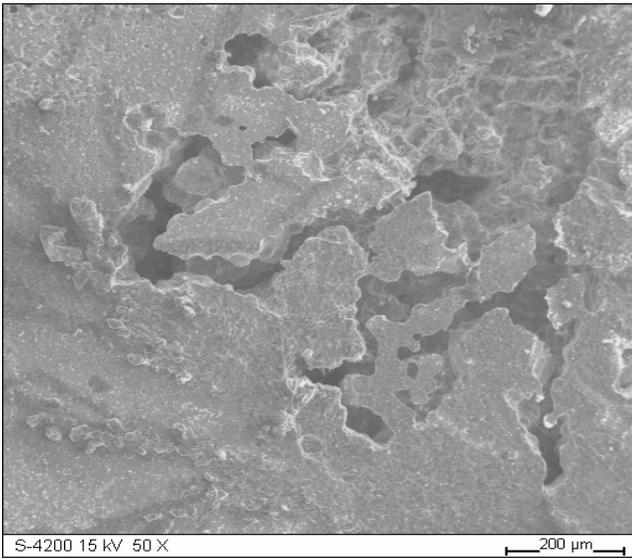
Fig. 5. Surface of Fe40Al5Cr alloy after corrosion tests in 3% H<sub>2</sub>SO<sub>4</sub> solution, scanning electron microscope, magn. 50x.
