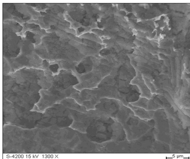
Fig. 3. Surface of Fe38Al alloy after corrosion tests in 3% H<sub>2</sub>SO<sub>4</sub> solution, scanning electron microscope, magn. 1300x.
