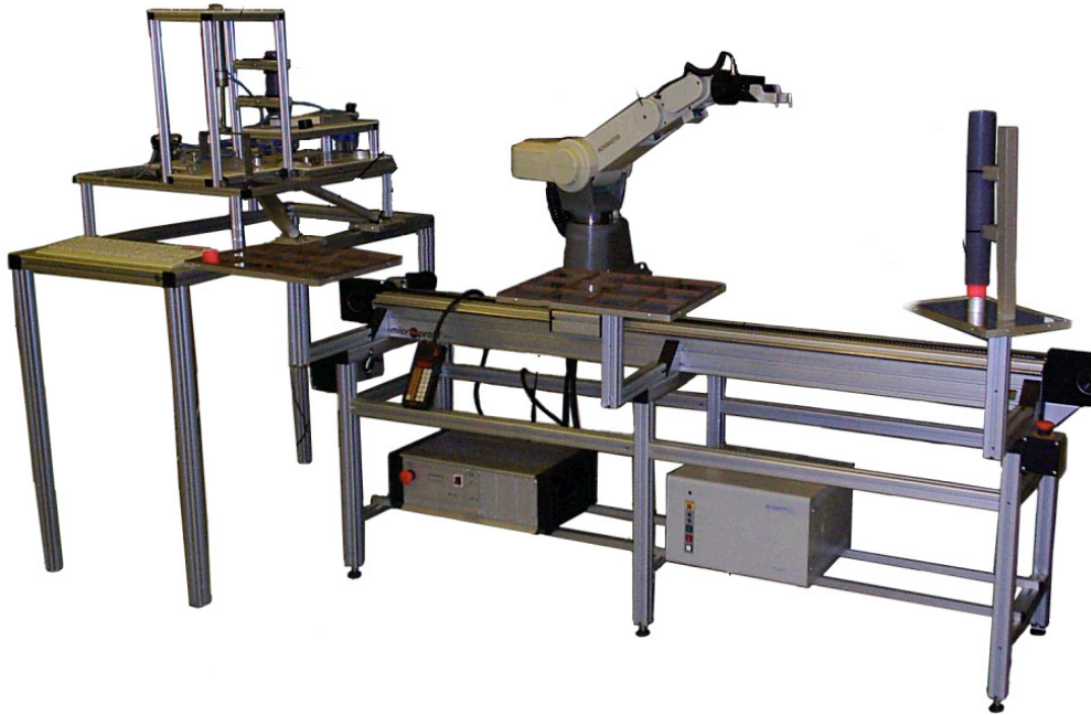
Fig. 9. Robotized laboratory stand with a colour separation module
