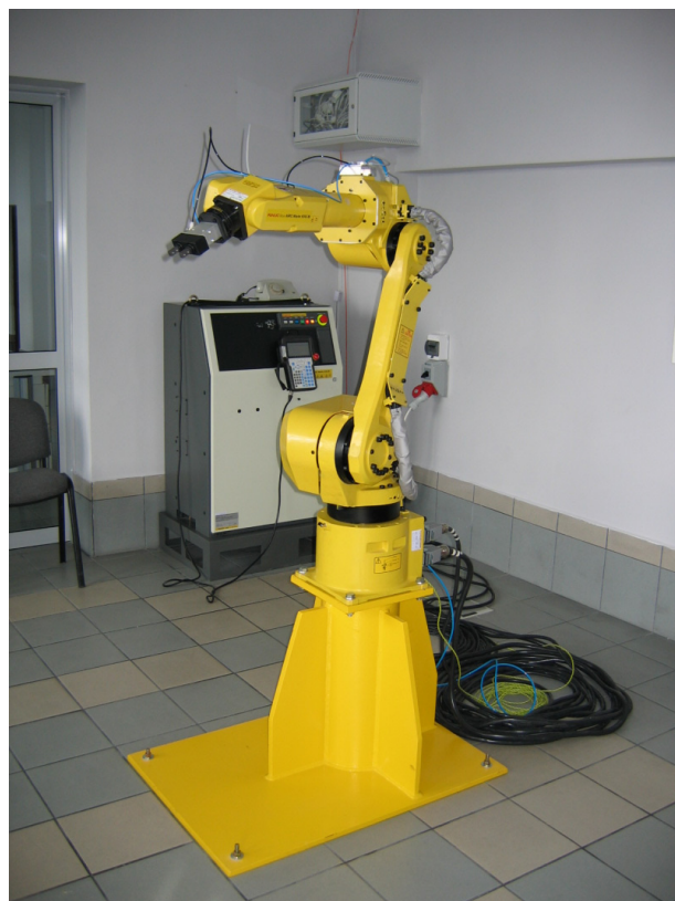
Fig. 8. Industrial FANUC robot intended for teaching of programming
