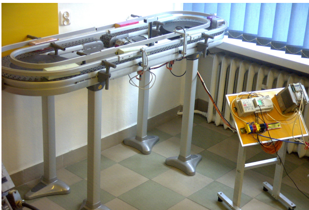
Fig. 13. Mechatronic system of flexlink belt conveyor-control based on mitsubishi frequency converters and ifm electronic sensory systems
