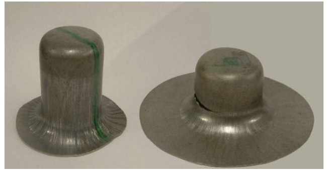
Fig. 17. Cups from a 100mm blank ( DR=3.1 ) when using the CPC heating technique (left) and the P one (right)
