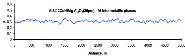
Fig. 3. The results of the friction coefficient value measurement for the friction couple: composite Al + intermetallic phases – composite AlSi12CuNiMg + 15% Al<sub>2</sub>O<sub>3</sub> (50μm), during cooperation under technically dry friction conditions
