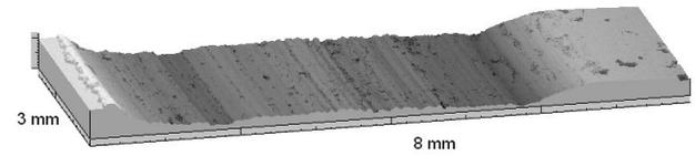
Fig. 5. Topography of the surface of AlSi12CuNiMg + 15% Al<sub>2</sub>O<sub>3</sub> (50μm) composite after cooperation with the composite Al + intermetallic phases under technically dry friction conditions
