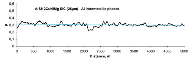
Fig. 6. The results of the measurement of the friction coefficient value for the friction couple: Al + intermetallic phases – composite AlSi12CuNiMg + 15% SiC (50μm), during cooperation under technically dry friction conditions
