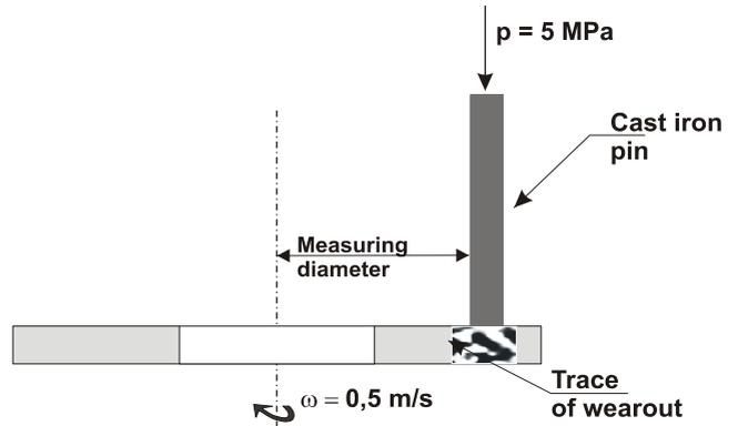
Fig. 2. Scheme of the pin-on-disc measuring system applied for the investigations of wear under technically dry friction conditions
