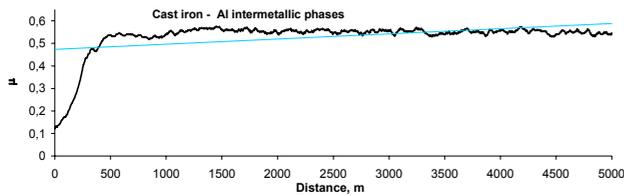
Fig. 9. The results of the measurement of the friction coefficient and wear values for the friction couple: cast iron – composite Al + intermetallic phases, during cooperation under technically dry friction conditions
