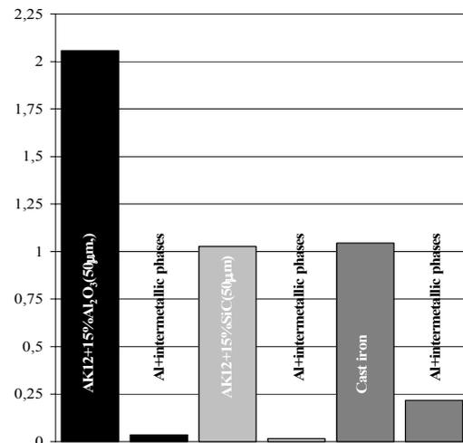
Fig. 12. Mass decrement of pins subjected to investigation under technically dry friction conditions
