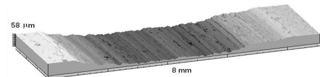
Fig. 8. Topography of the surface of AlSi12CuNiMg + 15% SiC (50μm) composite after cooperation with the composite Al + intermetallic phases under technically dry friction conditions
