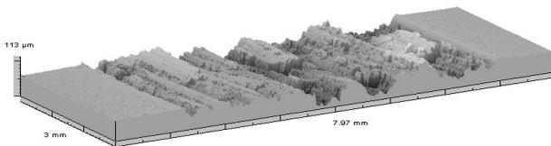
Fig. 11. Topography of the surface of composite Al + intermetallic phases after cooperation with spheroidal cast iron under technically dry friction conditions
