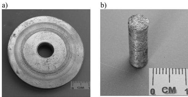
Fig. 10. View of the friction couple elements: a) disc – spheroidal cast iron, b) pin – composite Al + intermetallic phases
