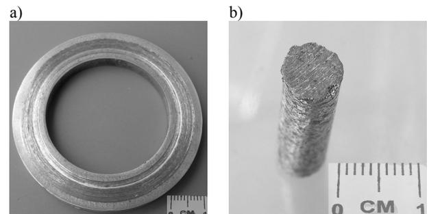
Fig. 7. View of the friction couple elements: a) disc – composite AlSi12CuNiMg + 15% SiC (50μm), b) pin – composite Al + intermetallic phases
