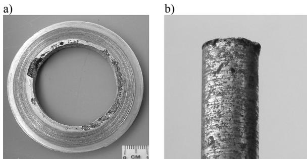
Fig. 4. View of the friction couple elements: a) disc: composite AlSi12CuNiMg + 15%Al<sub>2</sub>O<sub>3</sub> (50μm); b) pin – composite Al + intermetallic phases
