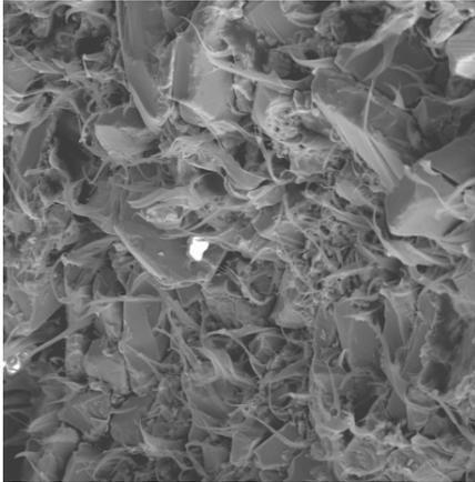
Fig. 4. Microscopic image of composite material fractures obtained after decohesion in the compression test – PEHD mass portion of 5.0% with powder  $\text{Fe}_{73.5}\text{Cu}_1\text{Nb}_3\text{Si}_{13.5}\text{B}_9$  alloy – milling time 0.25h – a) magnification 250x, b) magnification 500x
