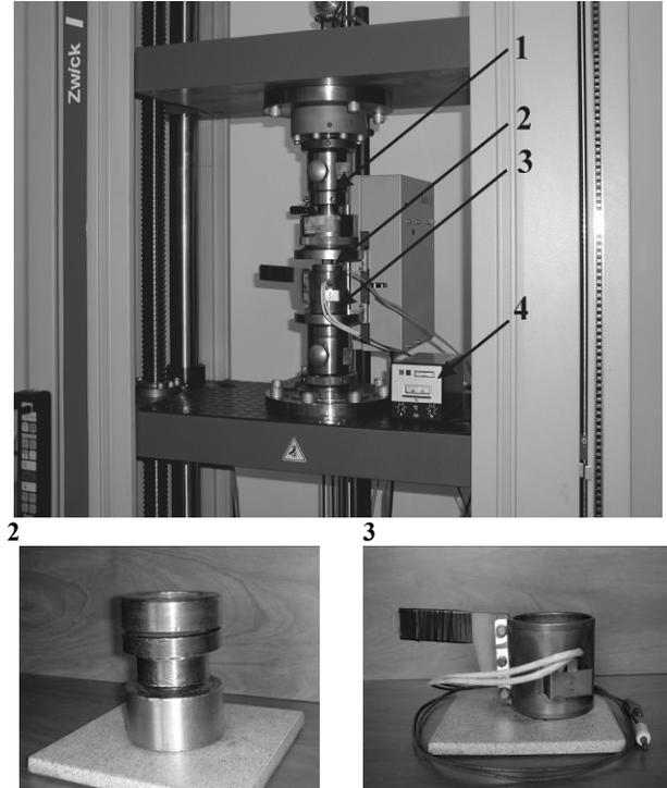
Fig. 3. View of the composite material forming stand: (1) testing machine set up for compression; (2) die block, (3) heater, and (4) thermometer
