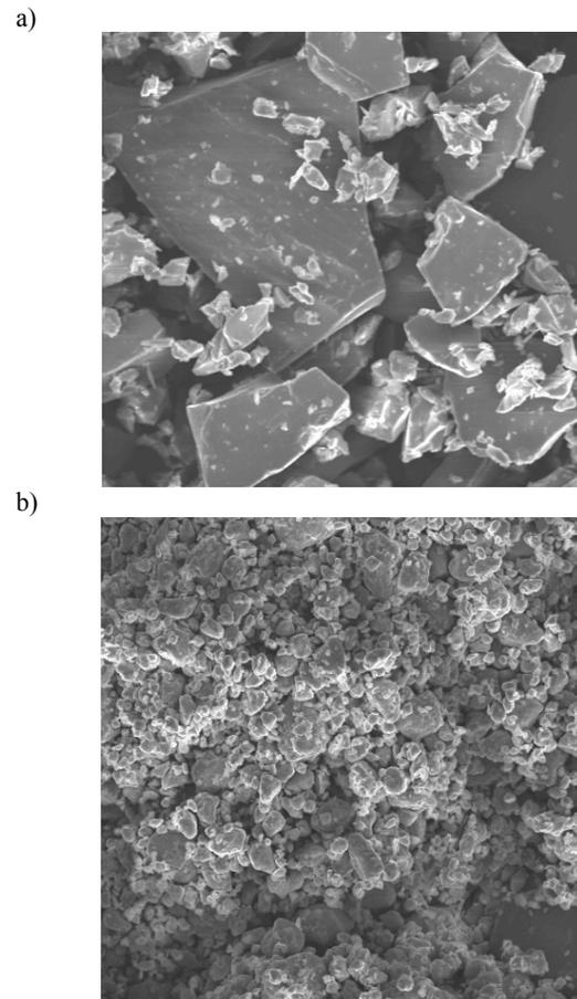
Fig. 1. The shape of  $\text{Fe}_{73.5}\text{Cu}_1\text{Nb}_3\text{Si}_{13.5}\text{B}_9$  powder particle – milling time: a) 0.25 h, b) 20.0 h (OPTON DSM scanning electron microscope - magnification 500x)
