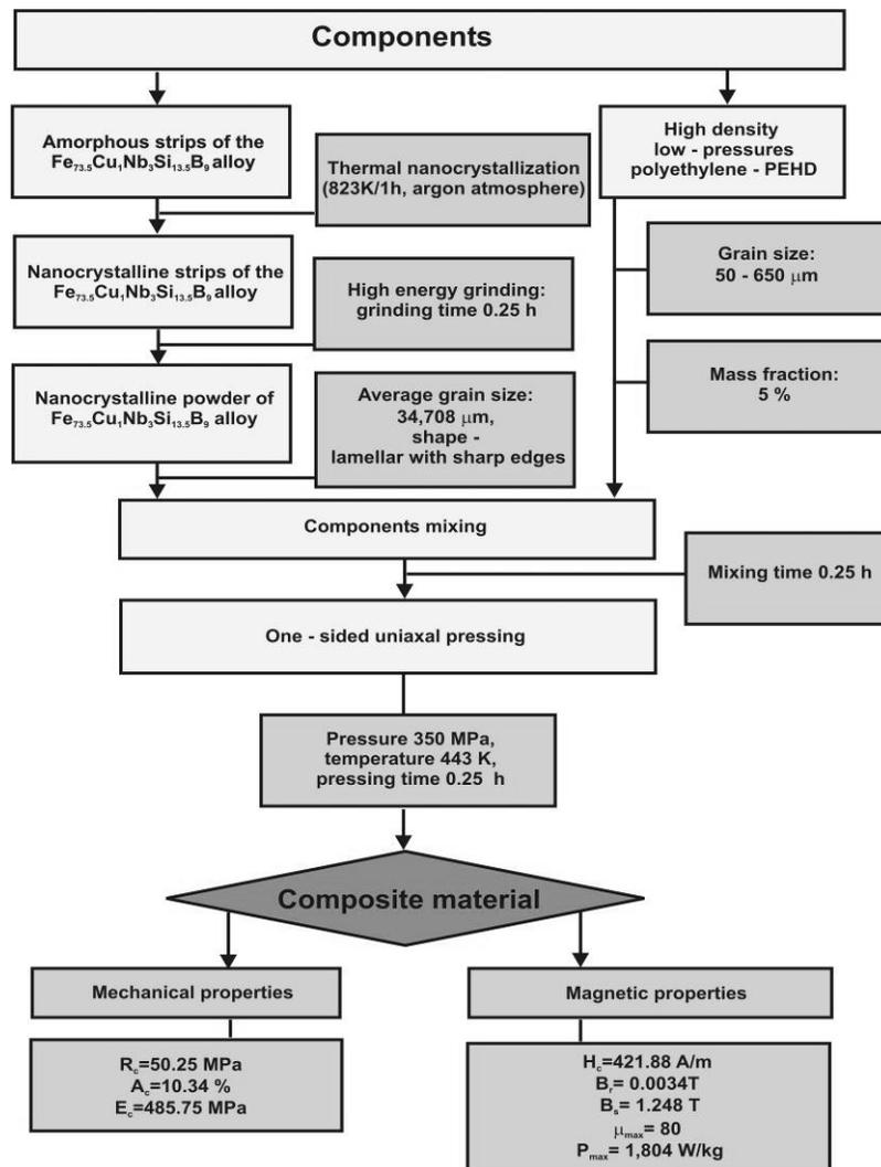
Fig. 5. Schematic diagram of the materials and technological operations for manufacturing the composite material with the most advantage combination of its mechanical and magnetic properties
