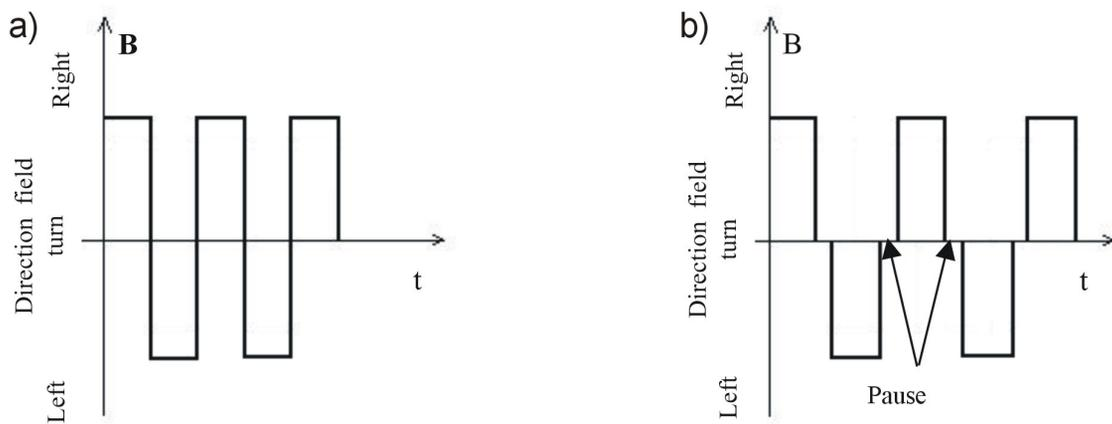
Fig. 2. Scheme of work cycles for reverse magnetic field (a) and impulse reverse magnetic field (b)
