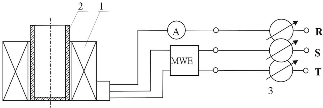
Fig. 3 Test stand scheme: 1- magnetic field coil, 2- mould, 3- three-phase transformer, A- ammeter, MWE- multivibrator
