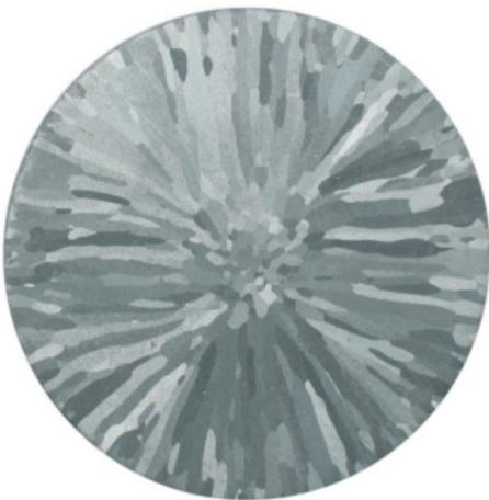
Fig. 6. Macrostructure of sample number 8  $f_p= 1$  Hz,  $I= 5$  A,  $M=75$  ppmTi+15ppmB
