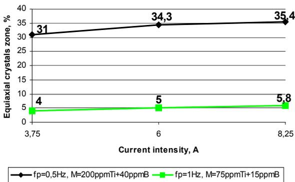
Fig. 11. Equiaxed crystals zone in function of current intensity
