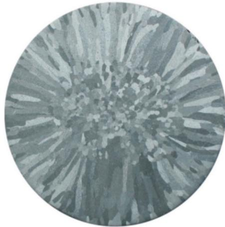
Fig. 8. Macrostructure of sample number 12  $f_p= 0.5$  Hz,  $I= 8.25$  A,  $M=100$  ppmTi+20ppmB
