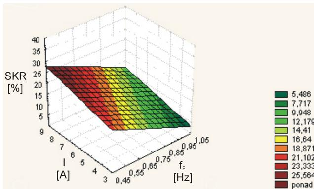
Fig. 12. Equiaxed crystals zone in function of current intensity and impulse frequency of magnetic field for identical quantity of inoculants (200ppm Ti + 40ppm B)
