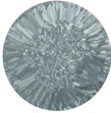
Fig. 7. Macrostructure of sample number 15  $f_p= 0.5$  Hz,  $I= 8.25$  A,  $M=200$  ppmTi+40ppmB
