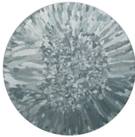
Fig. 9. Macrostructure of sample number 18  $f_p= 0.5$  Hz,  $I= 6$  A,  $M=200$  ppmTi+40ppmB
