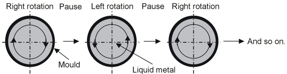
Fig. 1. Scheme of impulse reverse magnetic field influence on liquid metal
