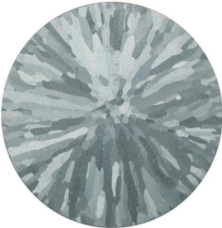
Fig. 4. Macrostructure of sample number 10  $f_p=0$  Hz,  $I=0A$ ,  $M=0ppm$  Ti+B
