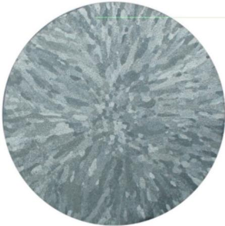
Fig. 5. Macrostructure of sample number 16  $f_p= 0$  Hz,  $I= 0$  A,  $M=200$  ppmTi+40ppmB
