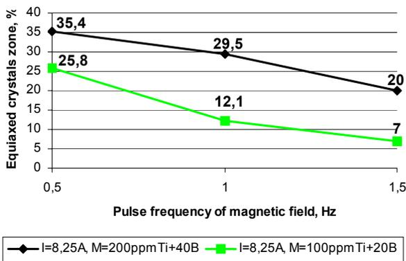
Fig. 10. Equiaxed crystals zone in function of pulse frequency of magnetic field
