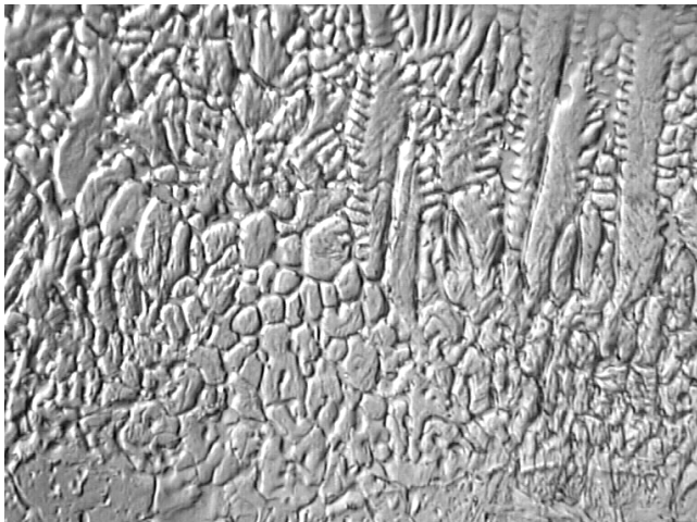
Fig. 3. The structure of surface layer after alloying by a HPDL laser; dendrites morphology of alloyed area; travel speed – 0,5m/min, laser power – 1,1 kW, thickness of the coating – 0,11mm (1000x)
