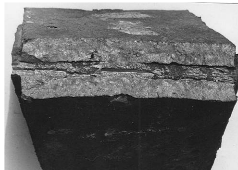
Fig. 16. Fracture of tested bimetallic casting
