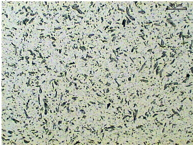
Figure 3. Microstructure of cross section of composite AA6061+15% Ti_3Al powder particle a) after 2h of L.E. mixing and b) after 18h of H.E. mechanical milling
