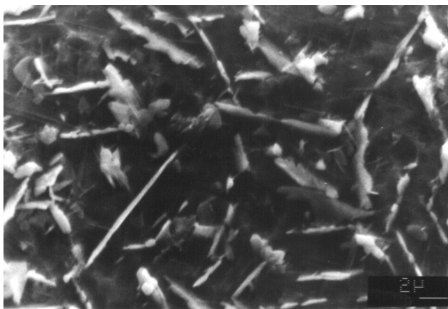
Fig. 9. Needle-shape particles of TiC and TiB phases in bottom part of alloyed zone
