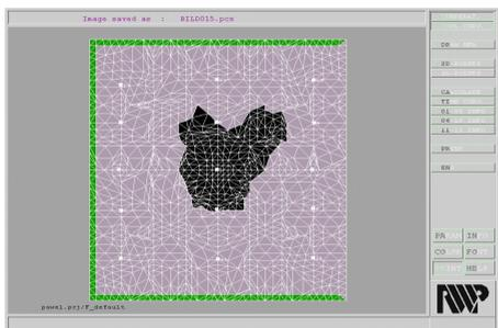
Fig. 2. Examples of micro - regions geometry containing single particle - created for simulation reasons. In figures geometry for real particles is shown: a) SiC, b)  $\text{Al}_2\text{O}_3$
