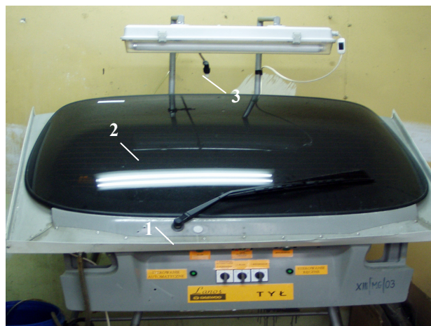
Fig. 4. Picture of the stand for evaluation of exploitation behaviour of car windshield wipers (see the text for figures)
