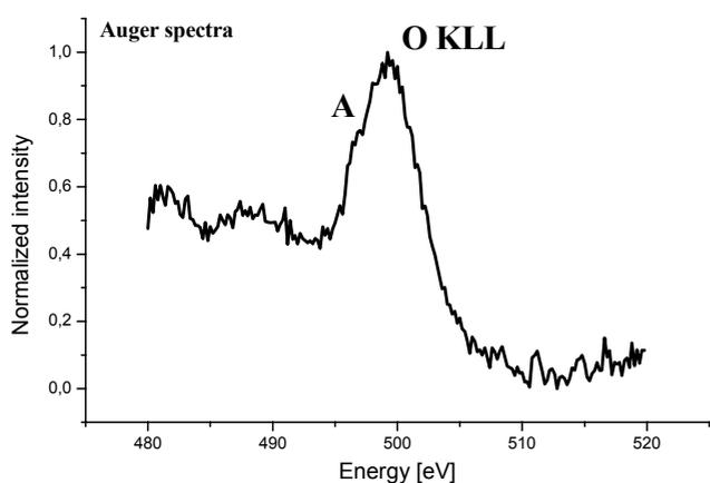
Fig. 4. Experimental shape of oxygen (KLL) and an additional (satellite peak A) Auger lines obtained for the Ni-Mo layers with polyethylene (Ni-Mo+PE) – 50 mA/cm<sup>2</sup>.
