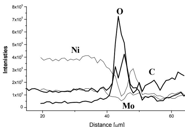
Fig. 5. Scan lines of the experimental intensities of the main Auger lines for elements Ni, O, Mo, and C obtained for Ni-Mo layers with polyethylene (Ni-Mo+PE) – 50 mA/cm<sup>2</sup>.
