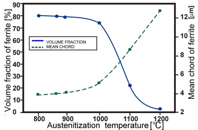
Fig. 15. Quantitative analysis of the volume fraction and mean chord of ferrite in the samples annealed at the various temperatures
