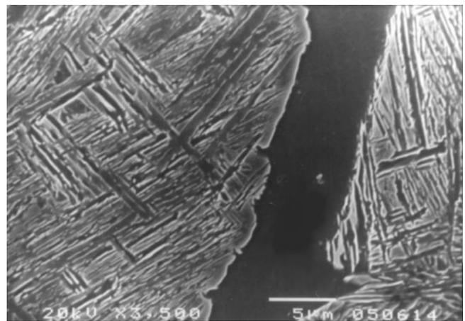
Fig. 7. Sample cooled from 1200°C/60s with the rate 40°C/s, SEM
