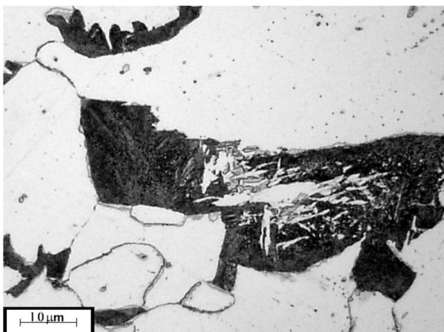
Fig. 10. Sample cooled from 1200°C/60s with the rate 0.5°C/s
