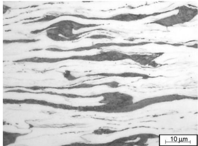
Fig. 3. The strip microstructure after cold rolling of the CMnAlSi steel
