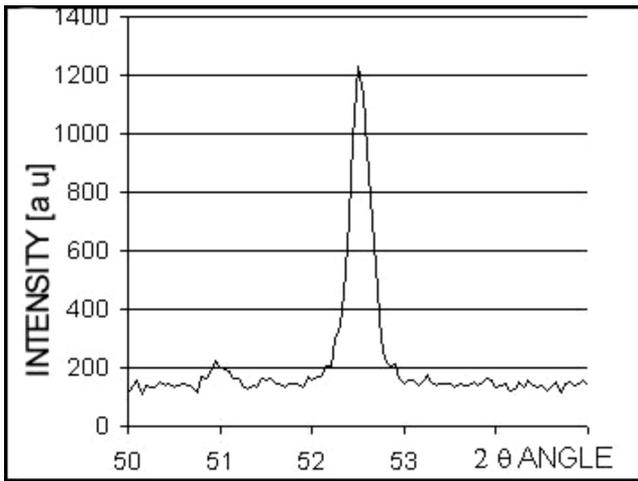
Fig. 20. X-ray diffraction of the sample heat treated according to the hot dip galvanizing line scheme (v)
