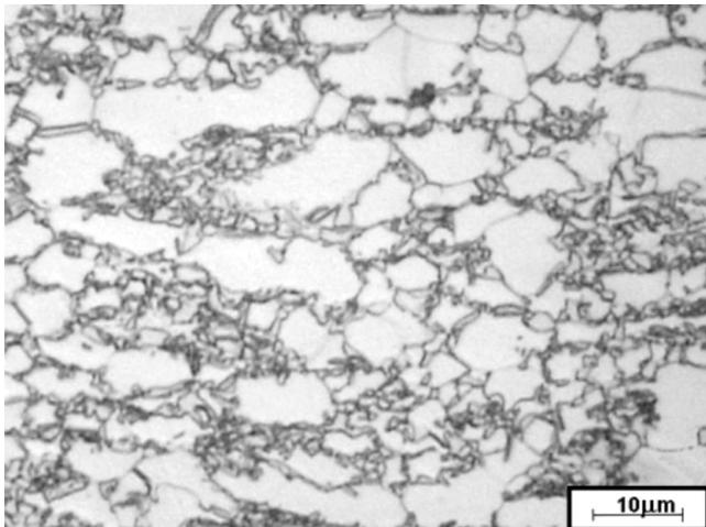
Fig. 16 . Typical TRIP microstructure of the investigated CMnAlSi steel
