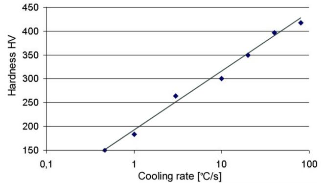
Fig. 21. Vickers hardness HV of the samples austenitized at 1200°C/60s, cooled with the various cooling rates, estimated from the Maynier's formula
