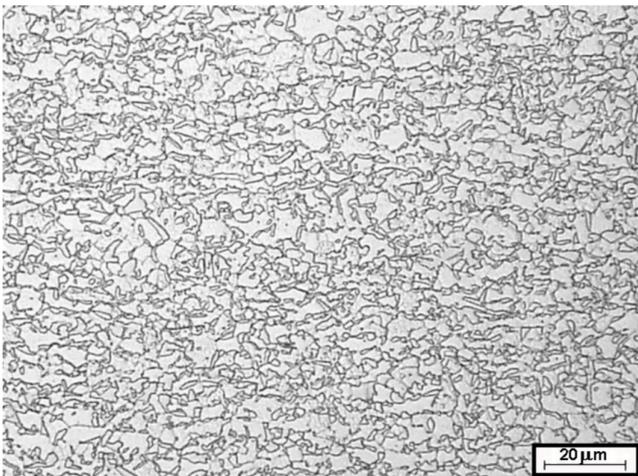
Fig. 14. Sample cooled from 900 °C/60s with the rate 20 °C/s
