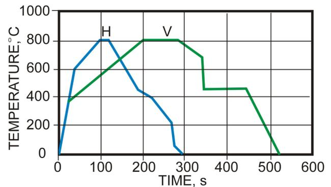
Fig. 4. Annealing cycles for vertical annealing (v)– hot dip galvanizing line and (h)-horizontal HDG line [1]
