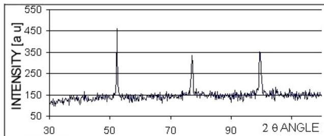
Fig. 19. X-ray diffraction of the sample in the initial state
