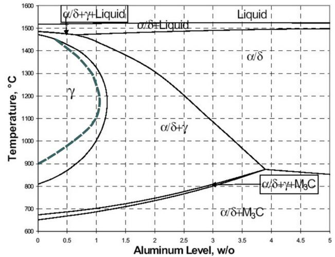
Fig. 5. Fe-0.1C-Al Phase diagram [10]
