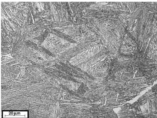
Fig. 8. Sample cooled from 1200°C/60s with the rate 40°C/s
