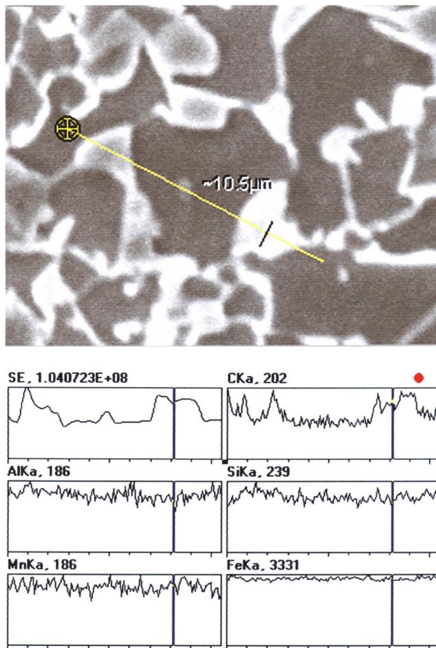
Fig. 18. Line chemical composition analysis of RA-TRIP steel
