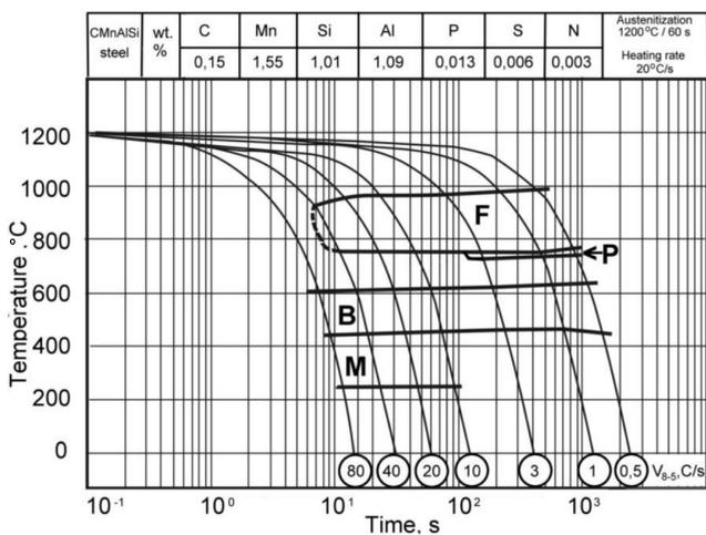
Fig. 6. CTPc diagram of the investigated steel austenitized at 1200°C/60s
