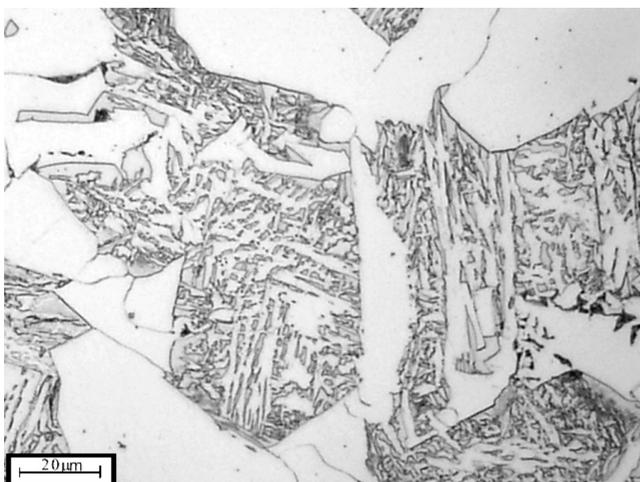
Fig. 9. Sample cooled from 1200°C/60s with the rate 3°C/s
