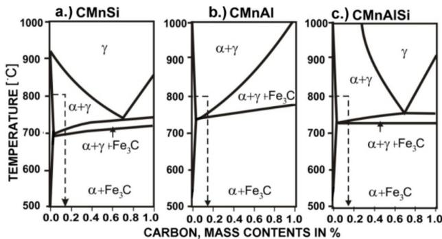
Fig. 2. Phase diagrams of CMnSi, CMnAl [2] and CMnAlSi steels after equilibrium calculations [3]
