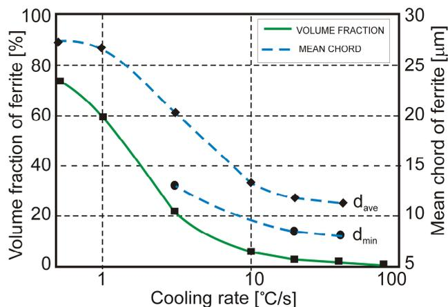
Fig. 11. Quantitative analysis of the amount of ferrite in the samples cooled with the various cooling rates
