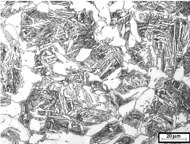
Fig. 12. Sample cooled from 1100 °C/60s with the rate 20 °C/s
