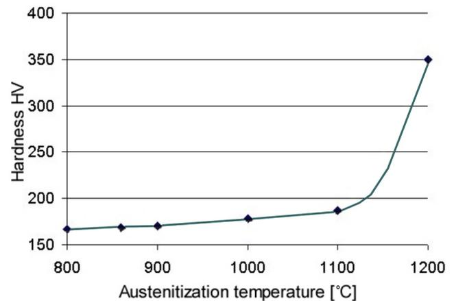
Fig. 22. Vickers hardness HV of the samples austenitized at various temperatures, cooled with the cooling rate 20°C/s, estimated from the Maynier's formula
