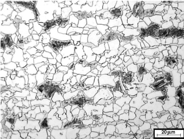
Fig. 13. Sample cooled from 1000 °C/60s with the rate 20 °C/s
