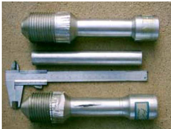
Fig. 6. The external and internal cylinders before testing and one specimen after bursting
